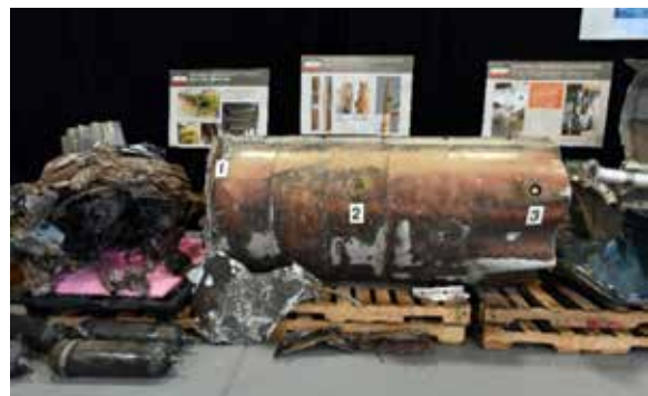
Debris from an Iranian Qiam SRBM provided by Iran to the Huthis that was fired into Saudi Arabia on display at Joint Base Anacostia-Bolling in Washington, DC. The numbered placards identify the unique positioning of valves on the missile's propellant tanks.
