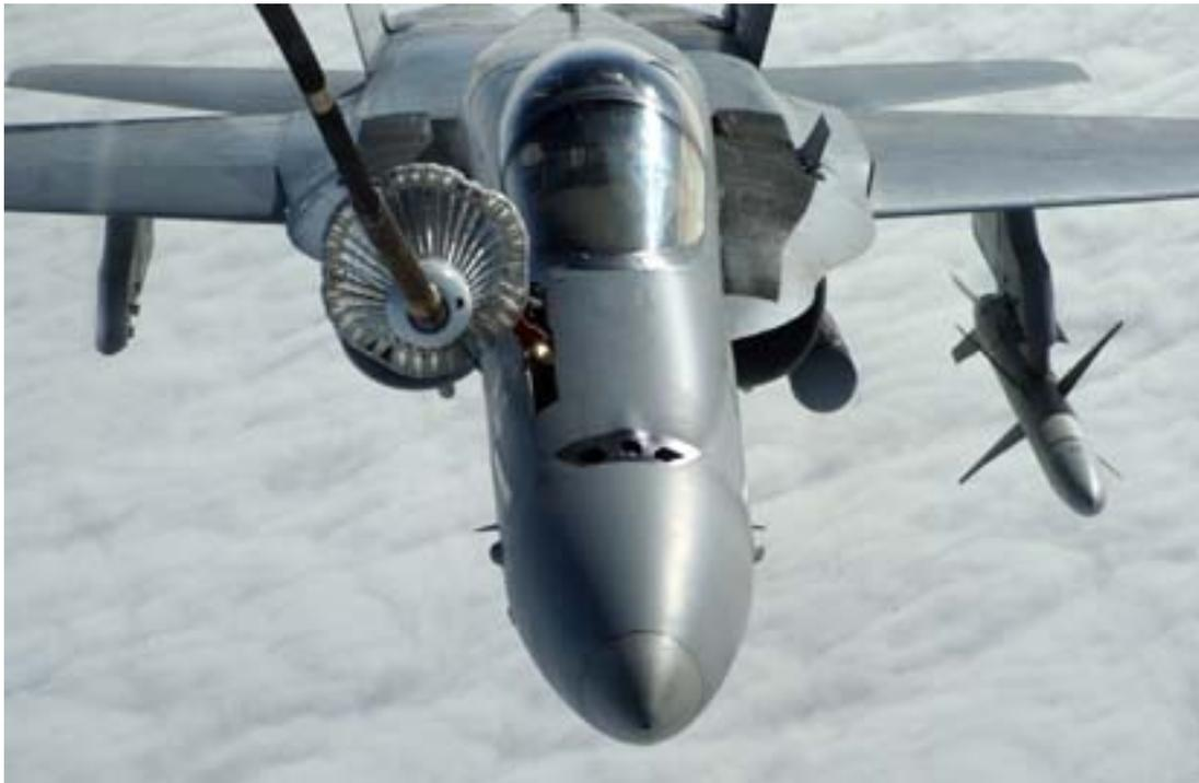
*United States Marine Corps F-18 receiver aircraft using drogue air refueling procedures.*
