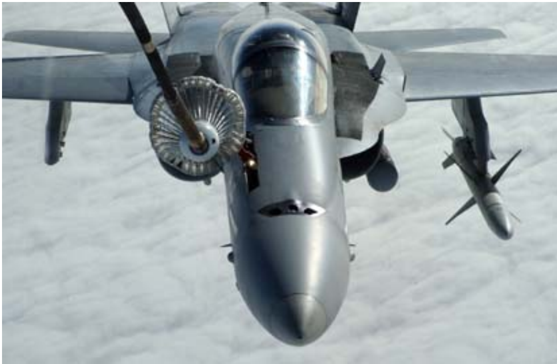
United States Marine Corps F-18 receiver aircraft using drogue air refueling procedures.
