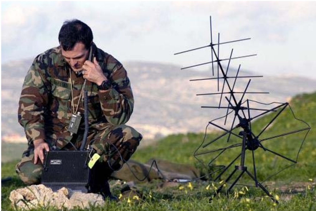
Portable satellite communications deployed to the field.
