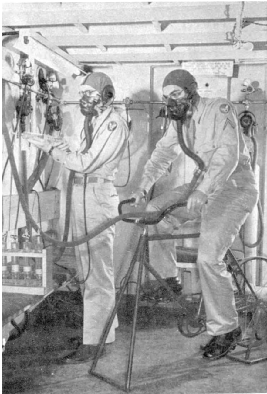
Simulating actual physical exertion of an airman in the sky, PFC. Asher J. Finkel, Chicago, pedals a wheel while wearing an oxygen mask. Lt. John T. Bonner, Rye Center, N. H., is checking the regulator to determine what mixture of oxygen and other gases is being given out by the apparatus, and to find out if the airman is getting enough oxygen from the present regulator.
