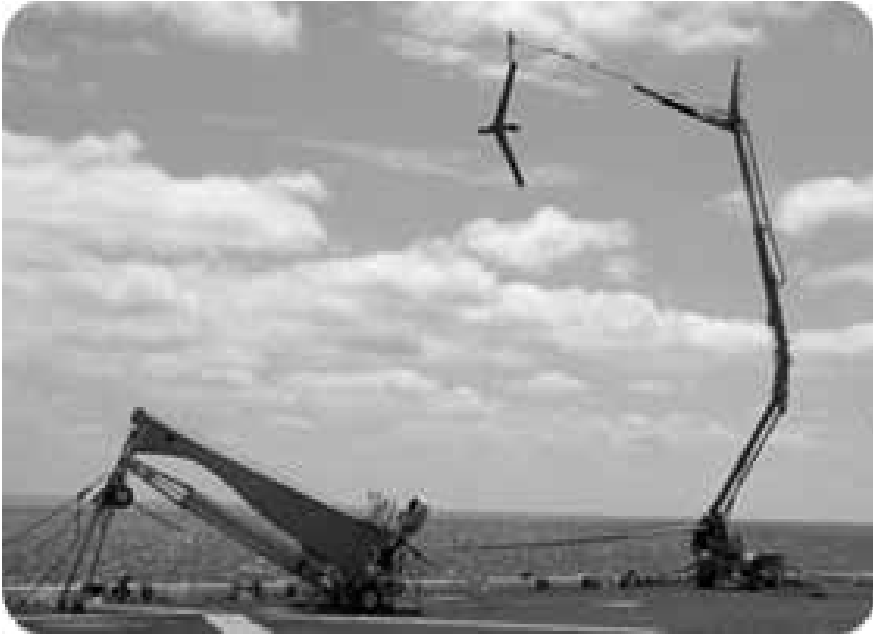
Figure 8. INSITU ScanEagle/Integrator launch and recovery system (Photograph courtesy of INSITU.)
