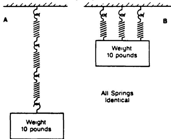
5. Ten-pound weights are each suspended from a ceiling by three identical springs. In A, the extension of each spring is
