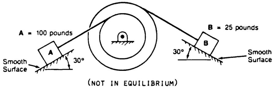
4. If weight B is to slide to the right, what change must be made in the diagram?
