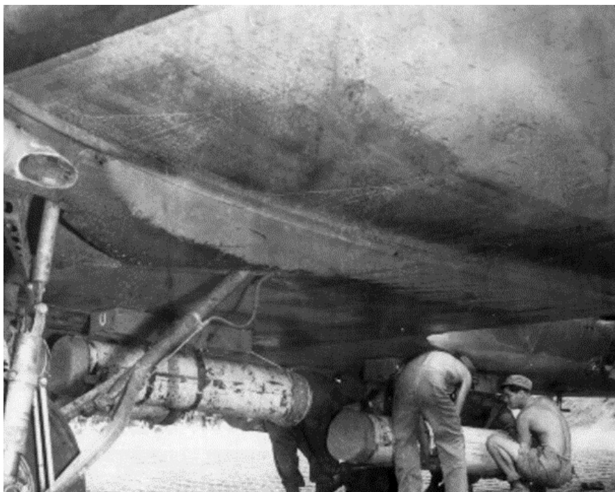
Figure 53. Royal Canadian Air Force personnel perform C-47 paracargo installation.
