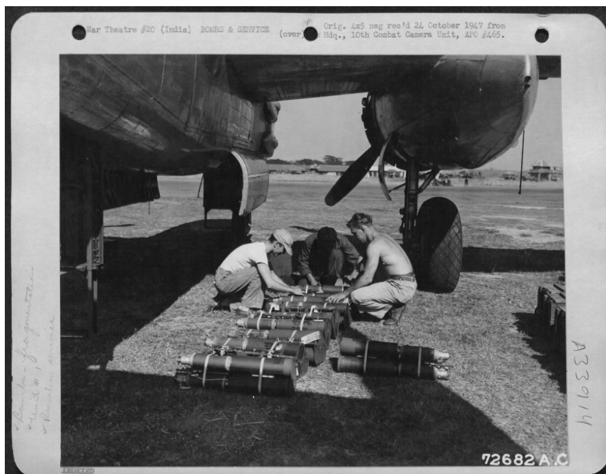
Figure 25. Ordnance personnel assemble bomb clusters for an Air Commando B-25, Chittagong, India, 23 January 1945.
