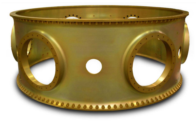
Fig. 26. This rendering shows an EELV Secondary Payload Adapter (ESPA) ring. (Image courtesy of Moog Inc.)
