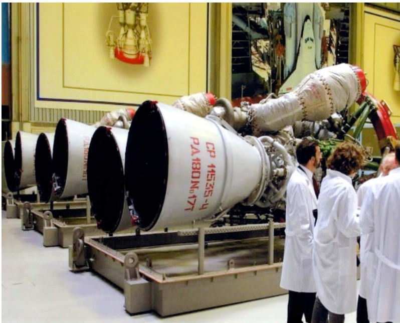
Fig. 23. Twin-nozzle RD-180 engines, manufactured by NPO Energomash in Khimki, Russia, are shown ready for shipment to United Launch Alliance (ULA) for the Atlas V, 6 June 2002. (Photo courtesy of John Hilliard)
