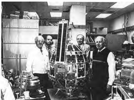
Figure 13-10. Poppy satellite with multiface design. (Photo taken by the NRL and provided courtesy of the NRO)
