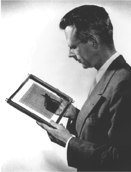
MIT's Jay W. Forrester, the inventor of the magnetic core memory, is shown holding a 64x64-digit memory plane. The plane was used in the Whirlwind/SAGE computer.
