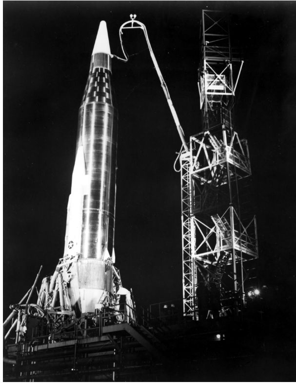
An Atlas ICBM topped with an ablative nose cone for a reentry test mission at the Air Force Missile Test Center.
