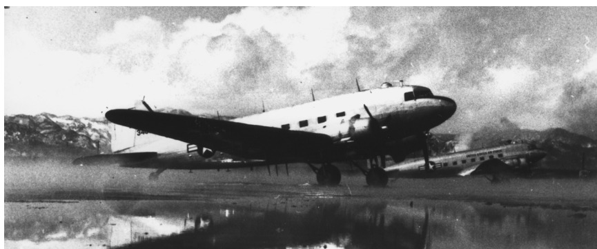
This C-47 is not quite what it appears to be. It was used by the 6147th TCG as an airborne radio relay aircraft.
