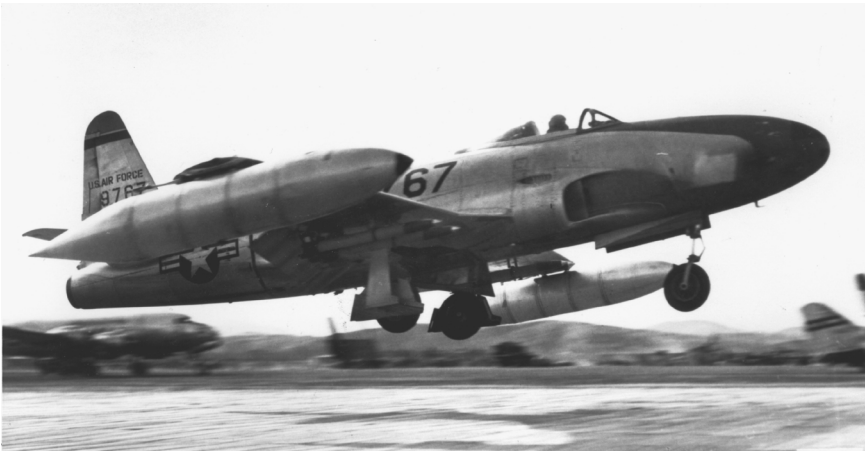
A rocket-armed F-80 takes off from a Korean airfield. It also carries the larger Misawa tip tanks.
