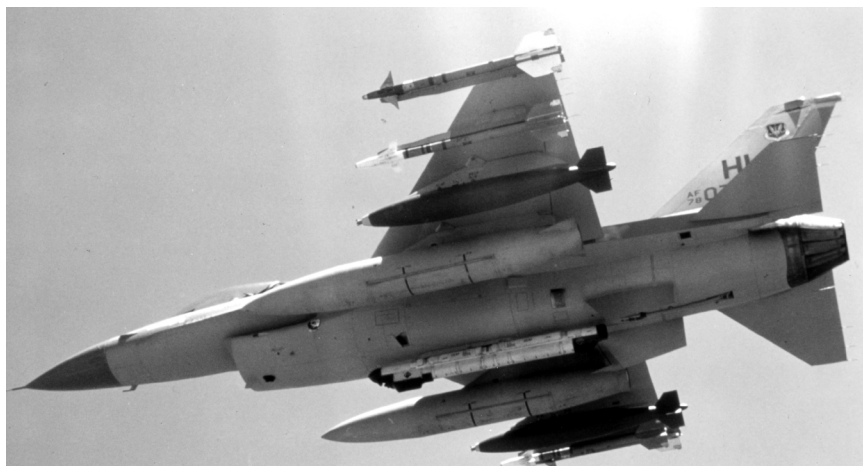
An F-16A of the 4th TFS (388th TFW) carrying a load of AIM-9L/M (on wingtips) and AIM-9P-2/3 Sidewinder missiles, a pair of MK-84 2,000-pound bombs, two 370-gallon drop tanks, and an ALQ-119 (V)-15 ECM pod. The 388th converted to the F-16C in 1989, flying this version during the Gulf War.
