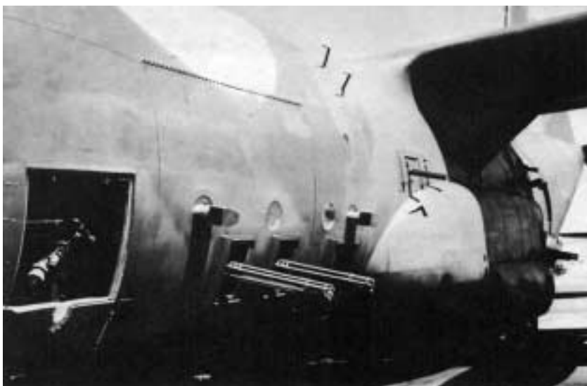
Miniguns and 20mm Vulcan cannons protrude from the side of an AC-130 gunship. This weapon system became the king of the truck killers along the Ho Chi Minh Trail.
