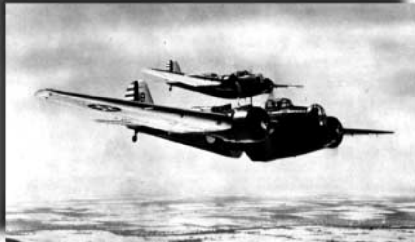
The Martin B-10 represented a new generation of bombers. It featured enclosed cockpits, a power-operated turret, and retractable landing gear.
