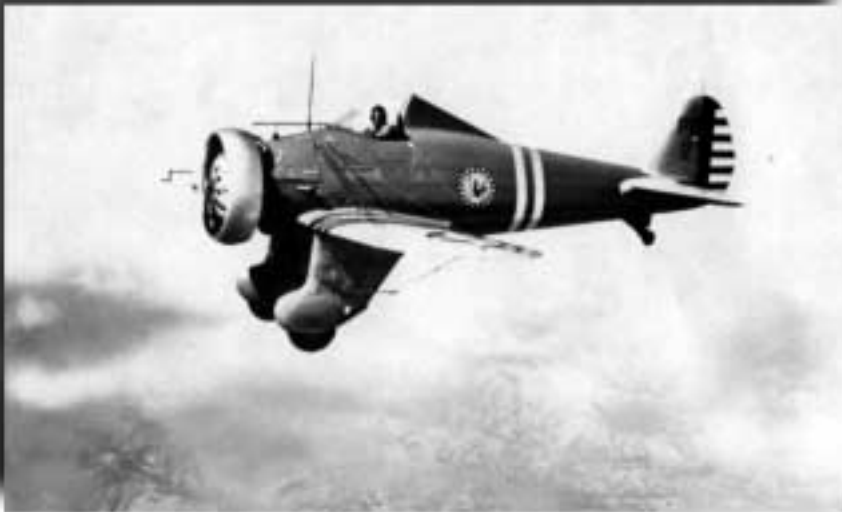
Designed to meet the increasing performance of the new bombers, the Boeing P-26 Peashooter was the first all-metal monoplane fighter built for the Army Air Corps.
