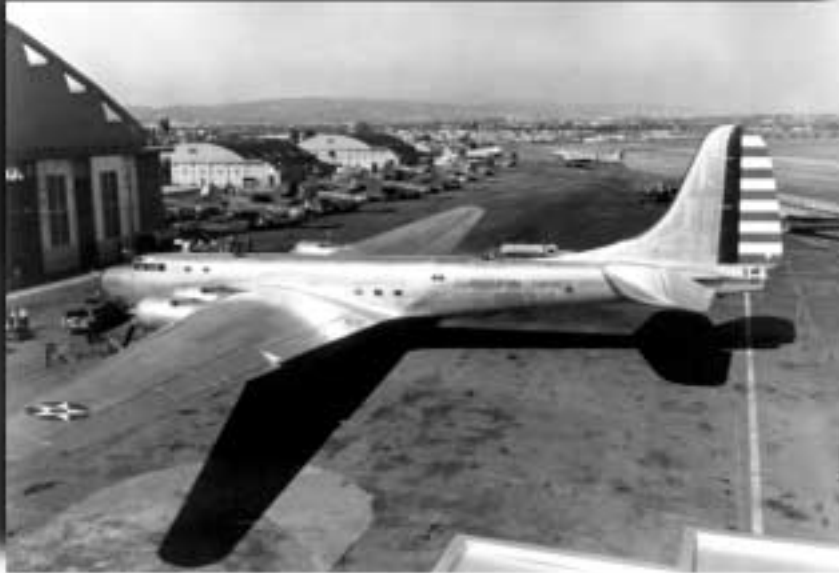
The Douglas XB-19, which first flew in 1941. With a wingspan of 212 feet, a 132-foot fuselage, and a rudder 42 feet high, it dwarfed other aircraft of its day.
