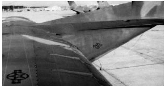
Horsal and dorsal fins were installed on Credible Sport to improve stability during low-speed flight.
