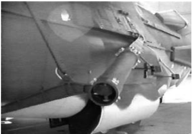
USAF Photo Eight Mark 56 rocket motors (four on each side) were mounted on the aft rear fuselage area and were pointed rearward at a 45-degree angle.
