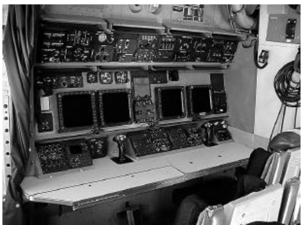
Nav/EWO panel on right side of Combat Talon II flight deck.
