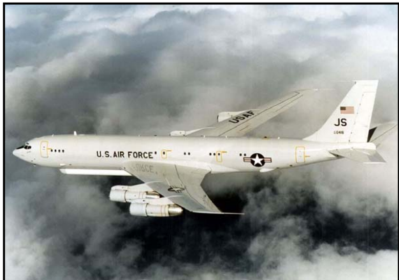
The JSTARS uses a multi-mode side looking radar to detect, track, and classify moving ground vehicles in all conditions deep behind enemy lines.
