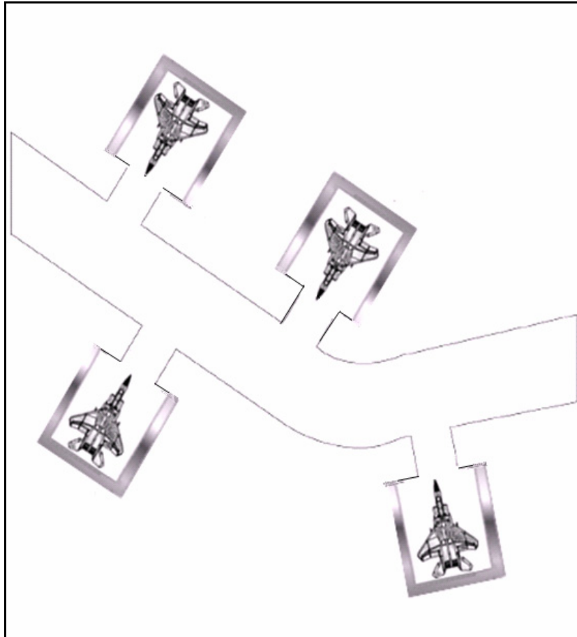
Figure 5.29. Dispersed Pattern for Aircraft Revetments.
