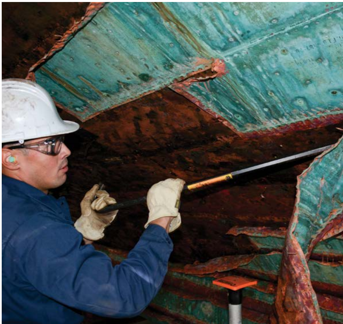
Seaman Jorge Ortiz, assigned to USS Constitution , pries a copper sheet away from the hull of Old Ironsides as a part of the restoration work being performed on the ship. Constitution is lined with 3,400 sheets of copper that are replaced every 15-20 years. U.S. Navy photo
