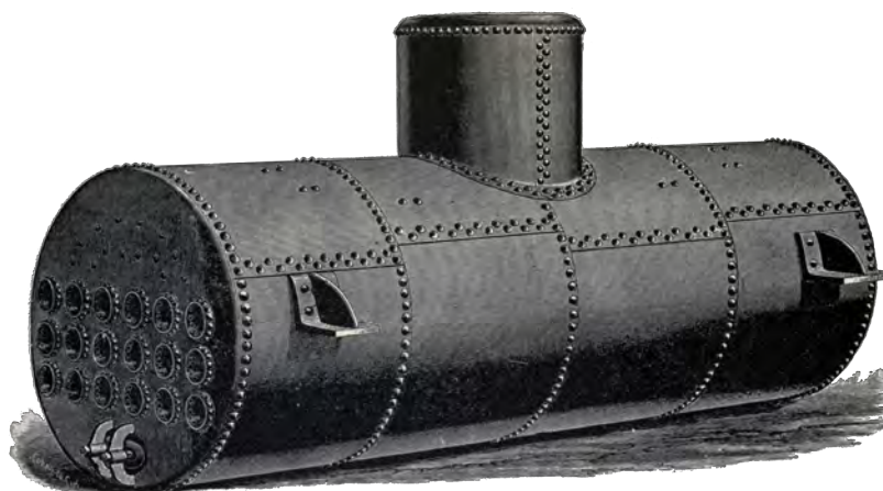
Figure 14.8. This flue boiler from Hutton (1897:443) provides an example of the number and position of rivets penetrating a typical boiler plate, making reuse challenging.
