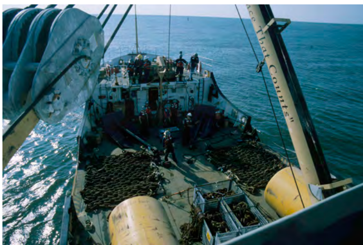
Figure 10.10. USCGC Madrona prepares to deploy the four mooring buoys used to secure Marks Tide safely without risk of damage to the site. (Courtesy of FOTH)
