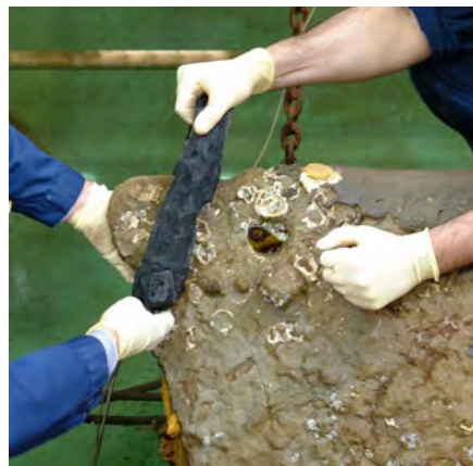
Figure 15.4. Project staff hold bracket HL-0526 against its hypothesized position on the submarine's bow casting. Note the square-headed fastener or nut for bracket HL-0582 immediately beneath the hole in the bow casting. (Detail of photograph by Susanne Grieve, courtesy of FOTH.)
