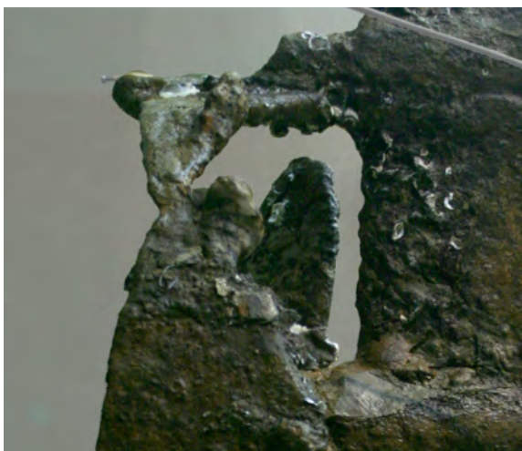
Figure 12.20. Damage to the top starboard quarter of the propeller shroud. (Photo by H. G. Brown, NHHHC).
