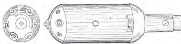
Figure 14.13. Drawing of a Civil War-era spar torpedo with multiple fuses distributed around a hemispherical head. (NHHHC Photo Archives #NH 59421)
