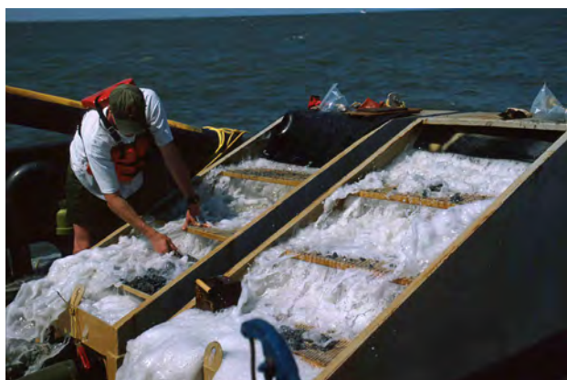
Figure 10.8. Sluice boxes designed by OII for screening dredge outflow had three tiers of increasingly smaller mesh. (Courtesy of FOTH)
