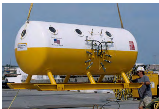
Figure 10.5. Hyperbaric chamber being readied for loading onto Marks Tide. (Courtesy of FOTH)
