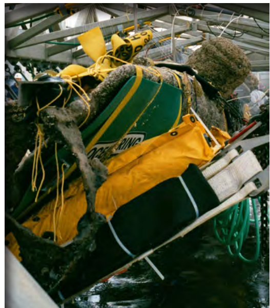
Figure 10.20. A patch was placed over the starboard stern hole to ensure no loss of interior contents. (Photo by Rand Pixa, courtesy of FOTH)
