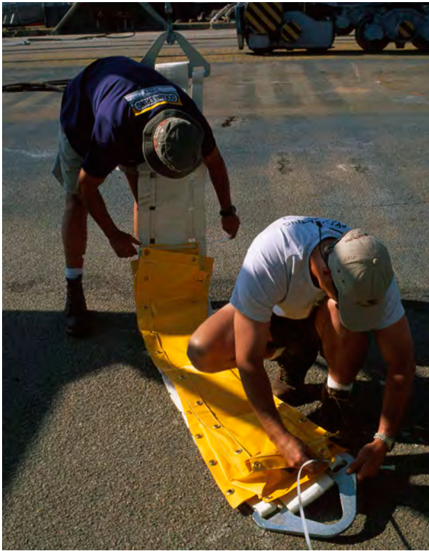
Figure 9.9. Members of the engineering team practice fastening a vinyl bag to a sling in land-based trials. (Courtesy of FOTH)
