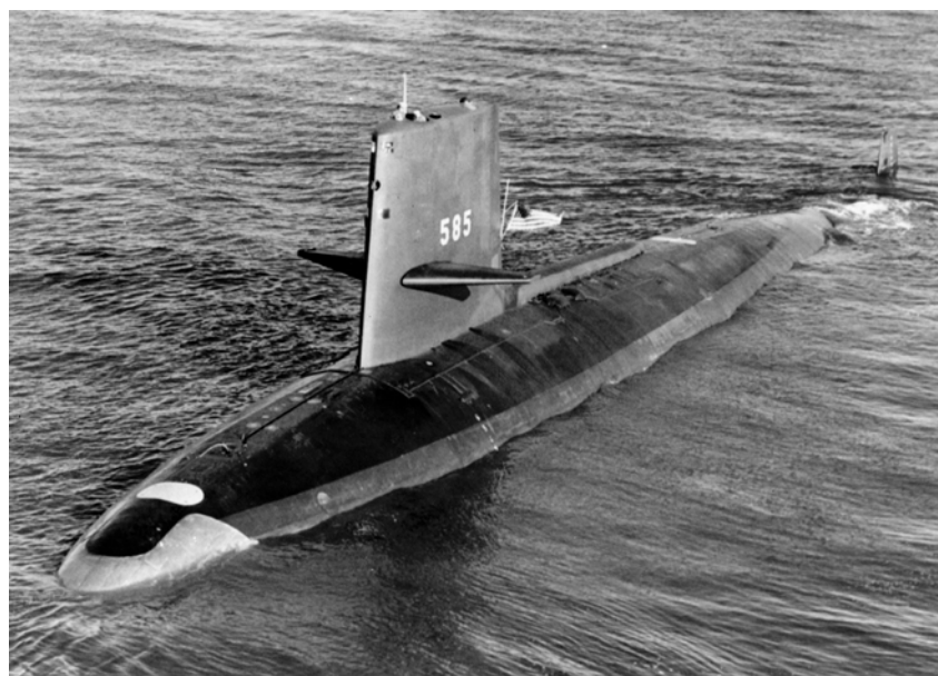
Figure 14.6. USS Skipjack (SSN-585) utilized a parabolic bow and gradually tapering body that is hydrodynamically ideal but costly to produce. (NHHC Photo Archives)
