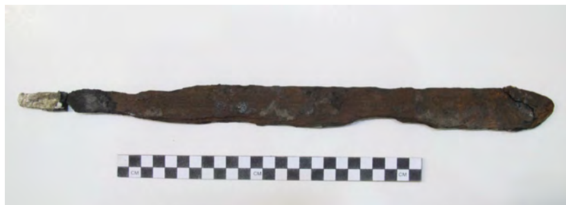
Figure 15.10. Cast of a wrought-iron bar (HL-0683) found near the rudder. (Photo by Virginie Ternisien, courtesy of FOTH)
