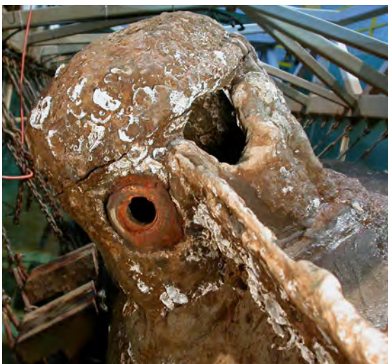
Figure 12.17. Hole in the forward conning tower encompassing the total loss of the port viewport (Courtesy of FOTH).
