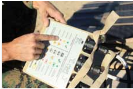
Gunnery Sgt. Andrew Suthers, the operations chief for the Infantry Officer Course in Quantico, Va., explains a color-coded light system on the Solar Portable Alternative Communications Energy System at the Combat Center Dec. 13, 2010. The SPACES is designed to tactically charge batteries and run communications equipment in remote areas such as Afghanistan. Photo: Sgt. Heather Golden
