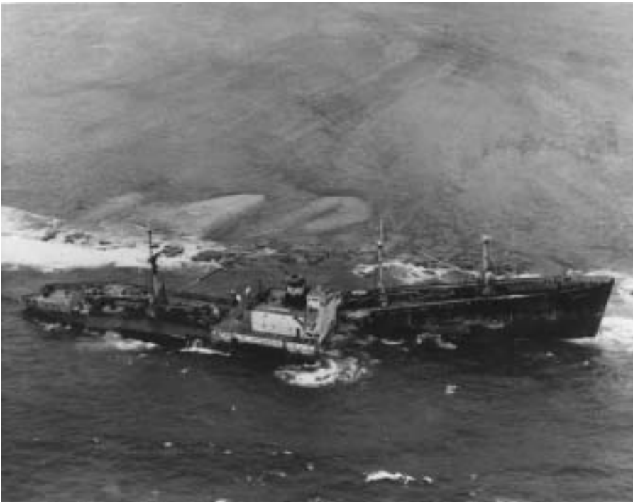
SS Quartette when first aground and after some time aground. The fate of Quartette vividly demonstrates the dangers of even the simplest grounding. Quartette was scarcely damaged in her initial grounding, but after some days' exposure to the force of the sea in conditions her designers never anticipated, she began to break up.
