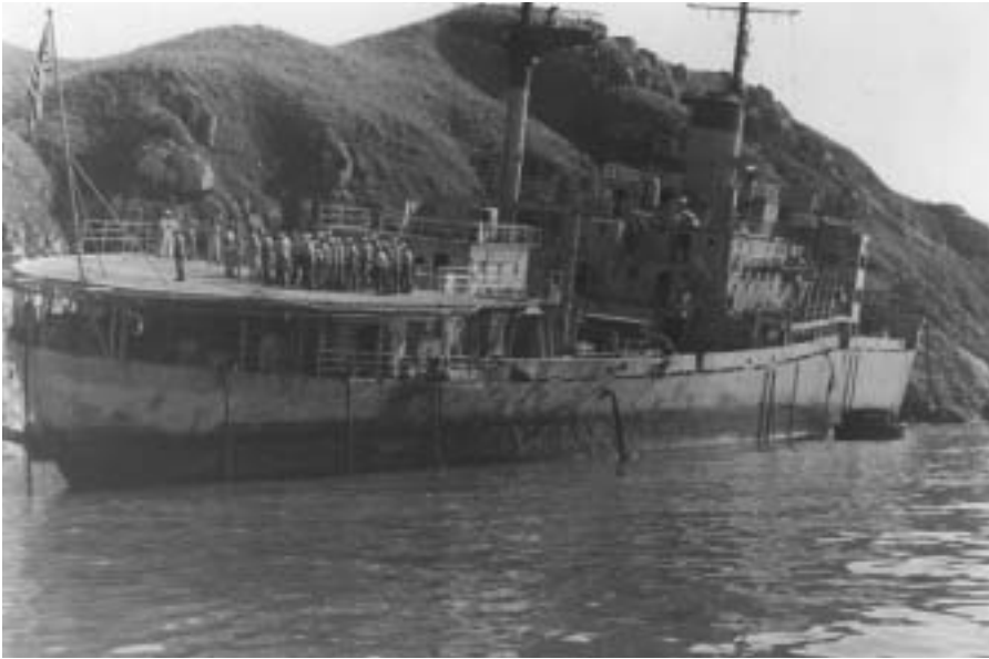
Regulus lies aground in Hong Kong harbor, showing the break in her hull caused by Typhoon Rose. Cut apart, her bow and stern were floated to a junkyard and sold.
