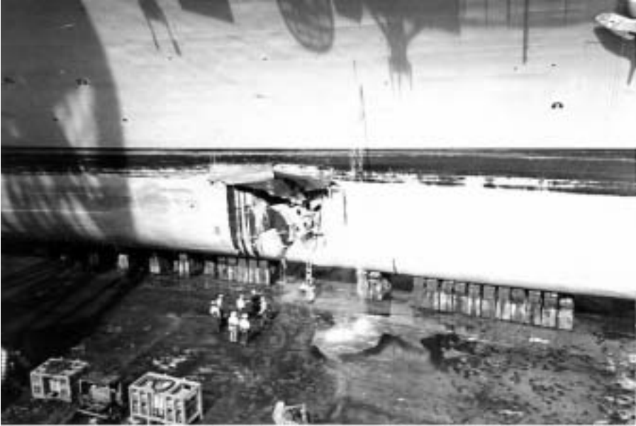
Mine damage on Tripoli's starboard side.
