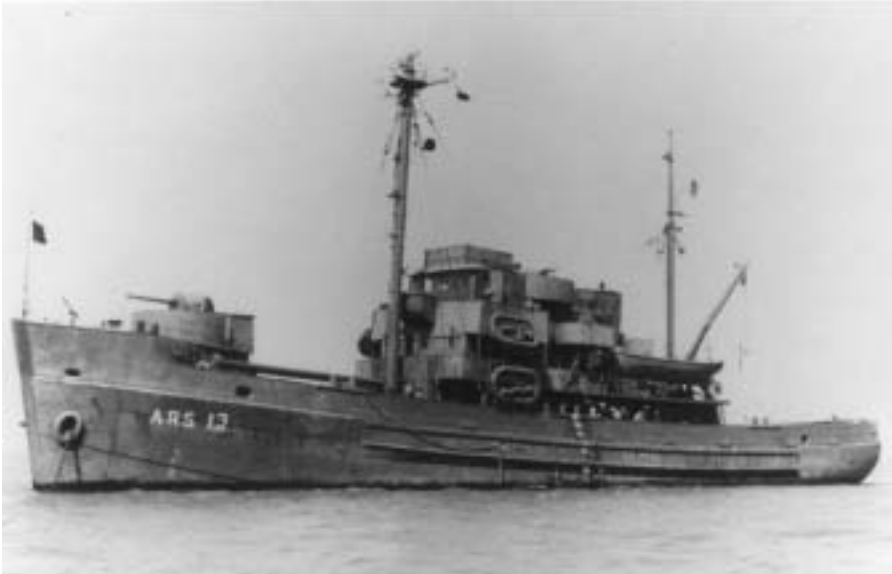
Anchor (ARS 13) was the class leader of a class of nine wooden-hulled salvage ships built during World War II. Note the absence of rollers for bow lifting.
