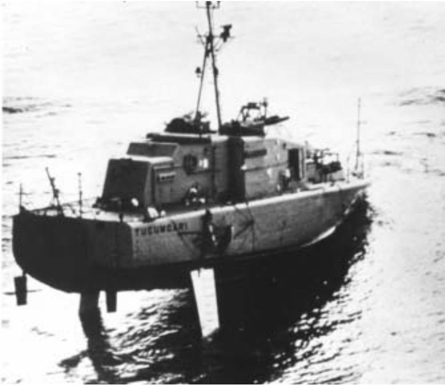
The hydrofoil Tucumcari , while flying on her foils, grounded off Puerto Rico in about 3 feet of water and ripped off her forward strut.
