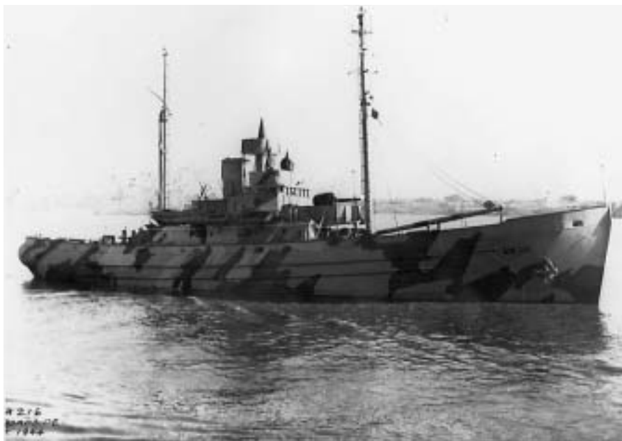
ATA-216, started as a steel-hulled net tender, was completed as a tug. She retains the rounded stern of the ATA.
