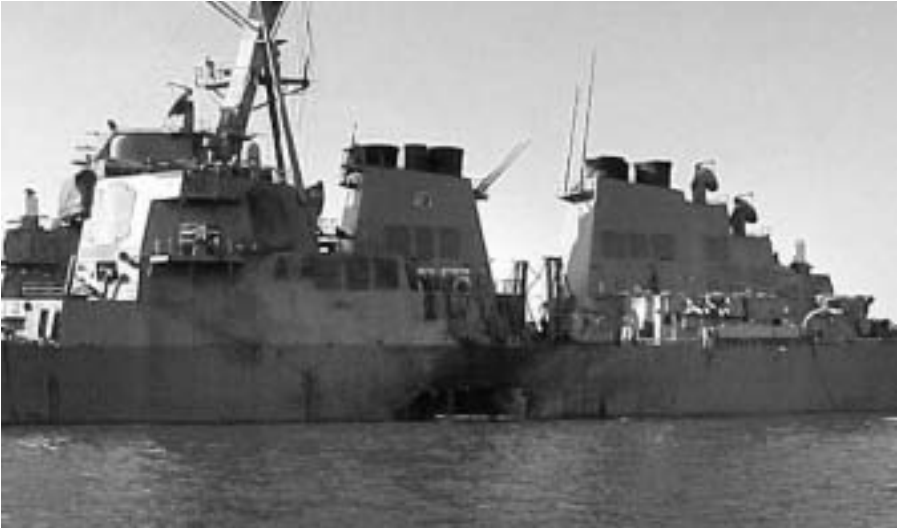
The port-side damage to guided missile destroyer Cole after a suicide bombing.
