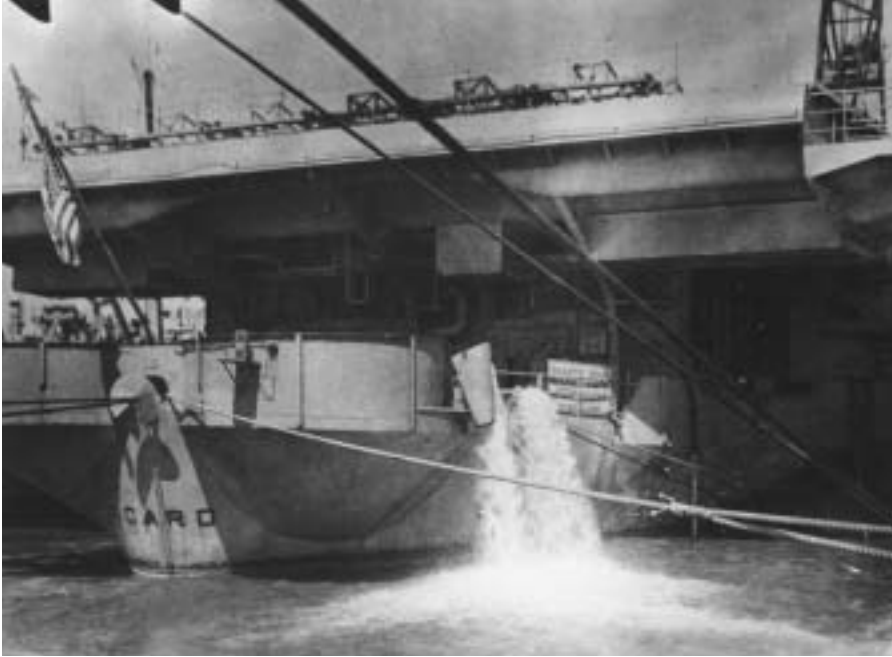
Water pours over the side as 6-inch submersible pumps discharge from USNS Card in Saigon.
