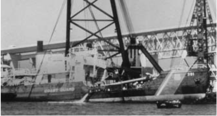
The 650-ton shear leg crane Cappy Bisso lifts the buoy tender Blackthorn from the waters of Tampa Bay, Florida.
