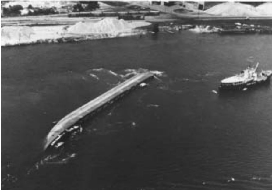
The Great Lakes ore carrier Sidney E. Smith lies capsized and sunk in the St. Clair River near Port Huron, Michigan. A bit later, the ship broke in two. Both sections settled into the bottom as the current, clearly visible here, scoured the bottom sand away.
