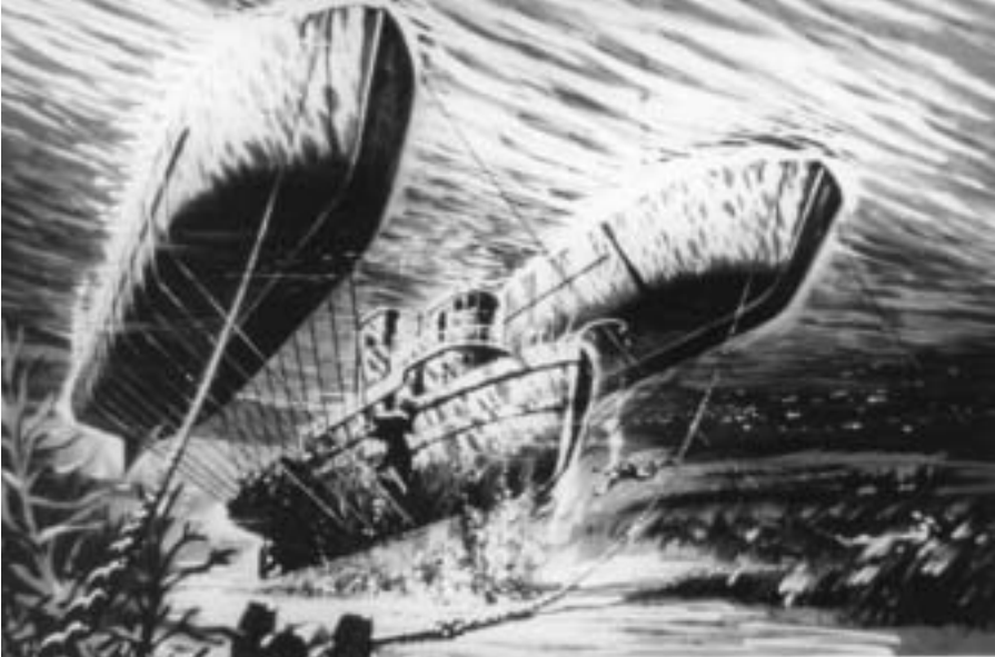
An artist's conception of Crilley and Crandall lifting the small tug Mogued in the Suez shows how the lift wires form a cradle to support the wreck.
