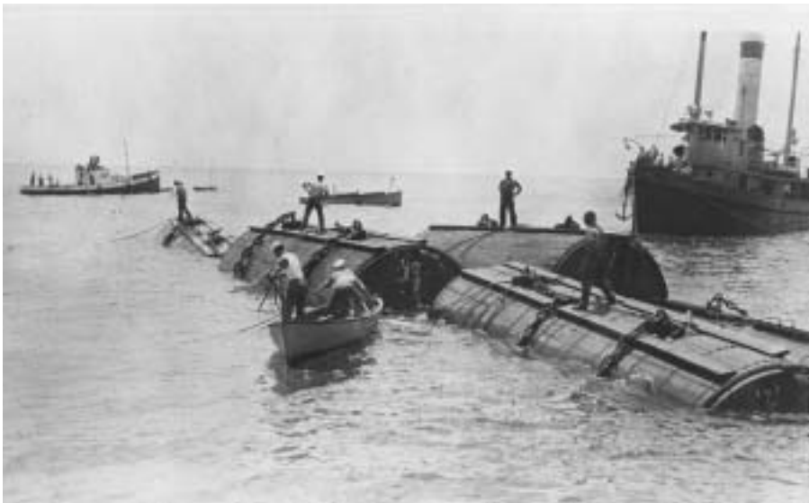
The final lift of the submarine F-4 was made using these submarine salvage pontoons designed by Naval Constructor Julius A. Furer.
