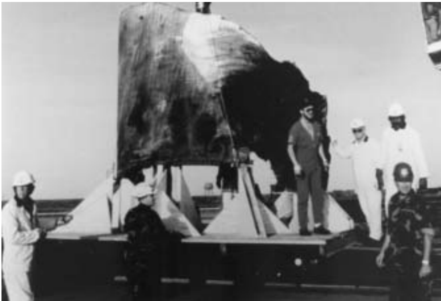
What it's all about: Recovery of this section of Challenger's right solid rocket booster with the burn hole allowed investigators to pin down the cause of the disaster.
