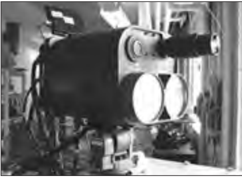
Laser Comms. NCST engineers and partners conducted laser communications experiments using hardware such as the Dual Mode Optical Interrogator and a test bed with facilities at the Chesapeake Bay Detachment (CBD) and at Tilghman Island, 16 kilometers across the Chesapeake Bay from CBD. 41
