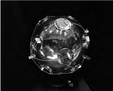
Space Reference. Launched on March 9, 1965, Dodecapole 1 served as a reference target for calibrating the Navy's Space Surveillance System (NAVSPASUR). Once in orbit, a mechanism involving twelve “trap doors” allowed metallic tapes to shoot out and form into 25-foot-long rods about 1/2 inch in diameter, resulting in a space target that was 50 feet across. (NRL photo 77112(14).jpg)
