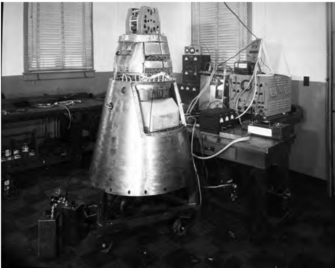
Science Warheads. To adapt captured V-2 rockets for upper atmosphere research, NRL engineers designed replacement warhead assemblies that could accommodate scientific instruments. Shown here are two NRL-made science “warheads,” including one in a laboratory where a cosmic ray telescope on the warhead is being tested for a March 7, 1947, launch. Forty-five Geiger-Muller counters and more than a half ton of lead were used in this experiment. (Top: Nosecone1_1947; “The Navy Upper Atmosphere Research Program With Rocket Vehicles, Part 1,” published on April 10, 1947; Bottom: NRL photo 60834(H-297))
