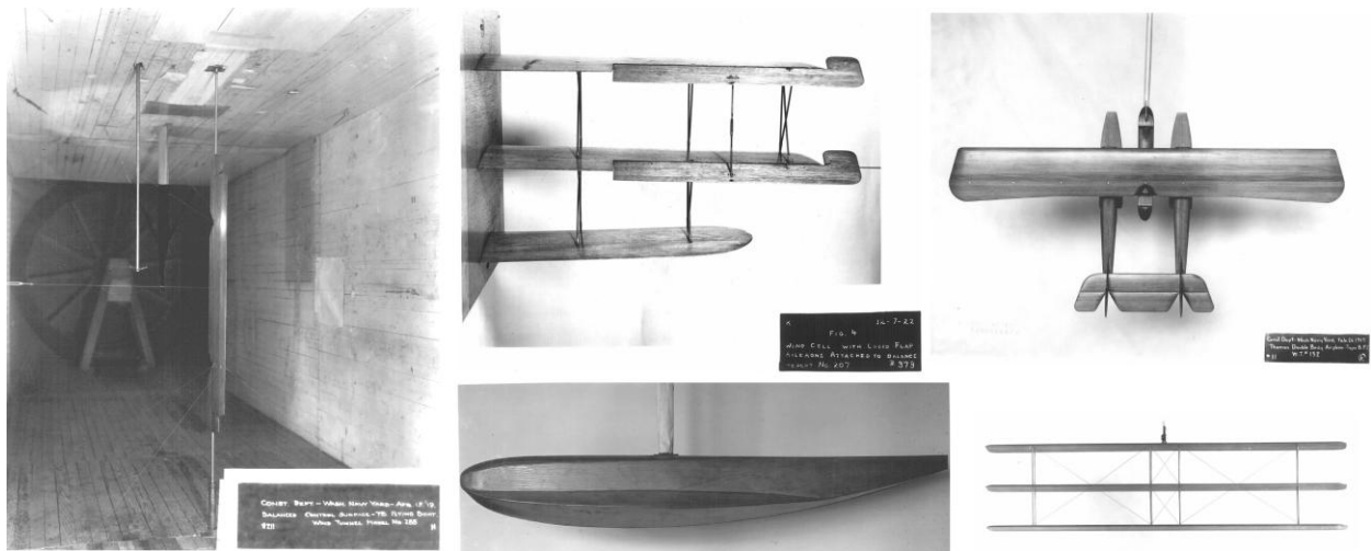
Figure 13. Numerous types of models were tested in the Navy's wind tunnel, including: isolated control surfaces (left), semi-span wing models (upper middle), and floats (lower middle), as well as full-span wing sets (lower right) and complete aircraft (upper right).
