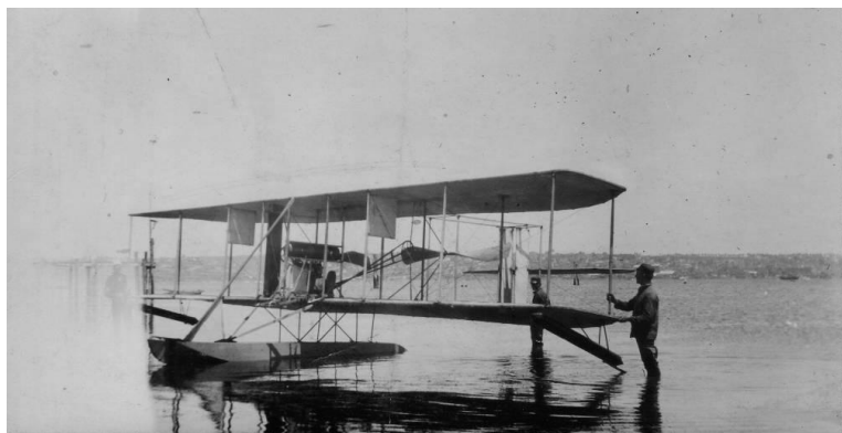
Figure 5. A Wright airplane was modified with floats for Navy evaluation.
