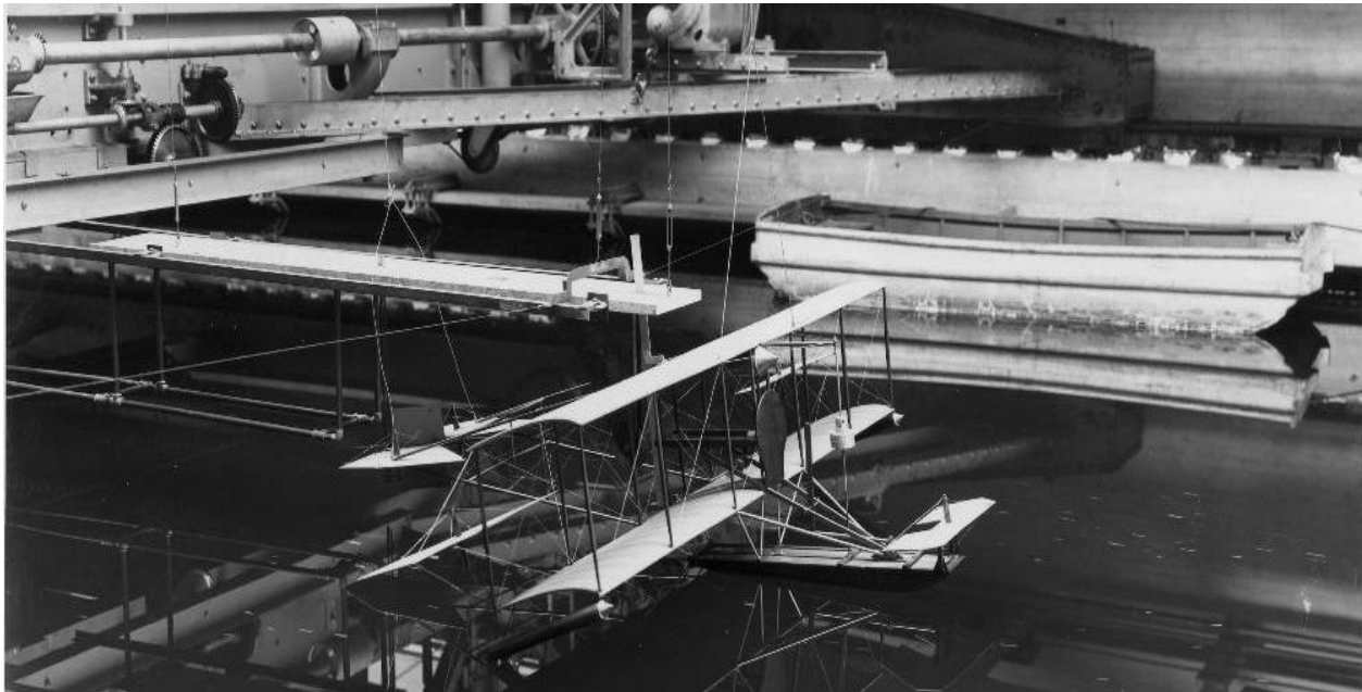
Figure 8. Testing of seaplane floats – and entire seaplanes – began in the Navy’s EMB in 1911 and led to greatly improved performance.
