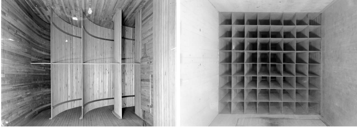
Figure 11. Vertical “splitters” (left) and a honeycomb grid (right) were incorporated into the wind tunnel to enhance flow quality.
