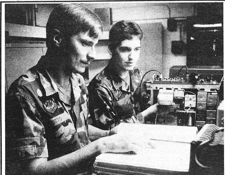
RADIO MAINTENANCE — SSgt. Raymond C. Otto, left, and SrA. John Galbraith, ground radio communications equipment technicians at the 1978th Communications Group, troubleshoot a frequency-modulated transceiver used by the Howard Air Force Base Command Post. (U.S. Air Force photo by SSgt. Debra L. Penton)
