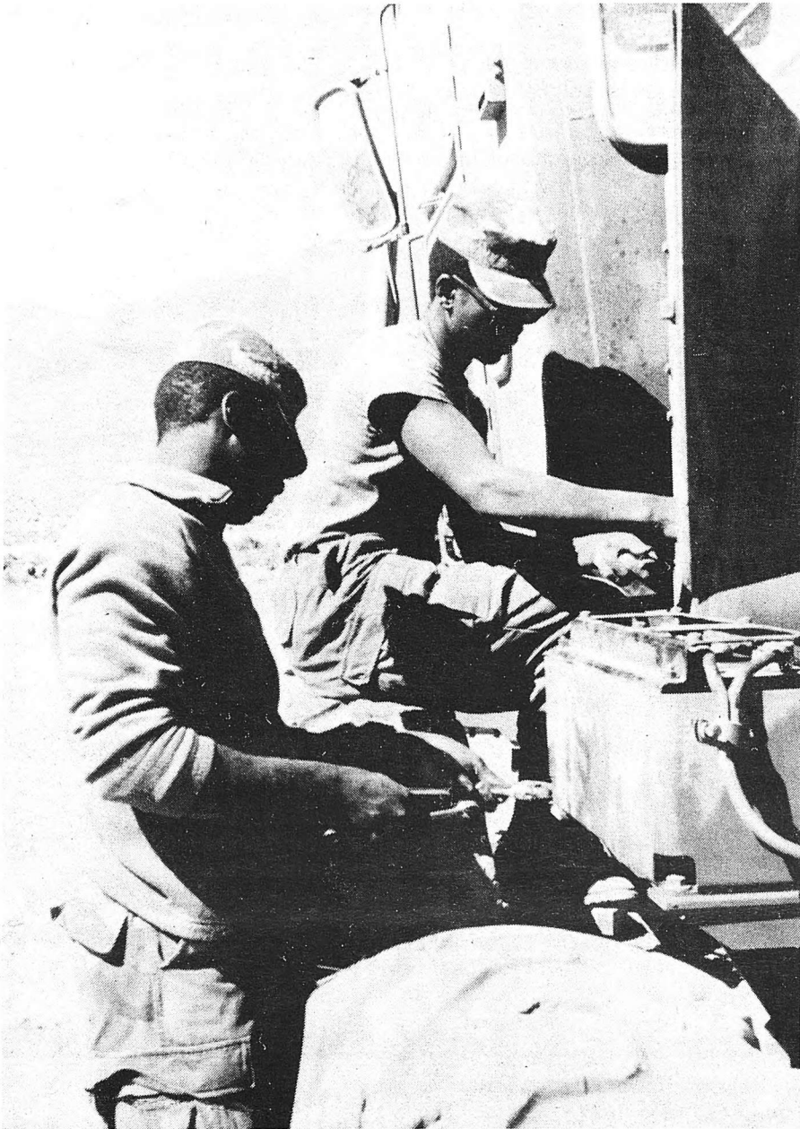
Spec. Yancey Caldwell (left) and Spec. Paul Burns, 15th Eng. Co., 536th Eng. Bn., Fort Kobbe, do brake repairs on a roadgrader. (U.S. Army photo by Sgt. Jon Connor)
