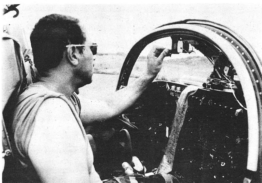
TSgt. Ray E. Martinet, 24th Consolidated Aircraft Maintenance Squadron, adjusts the compass on an OA-37 Dragonfly during a recent deployment for training exercise to Manta AB, Ecuador. It was one of six aircraft assigned to the 24th Tactical Air Support Squadron that were calibrated during the exercise. (U.S. Air Force by SSgt. Matthew Gildow)
