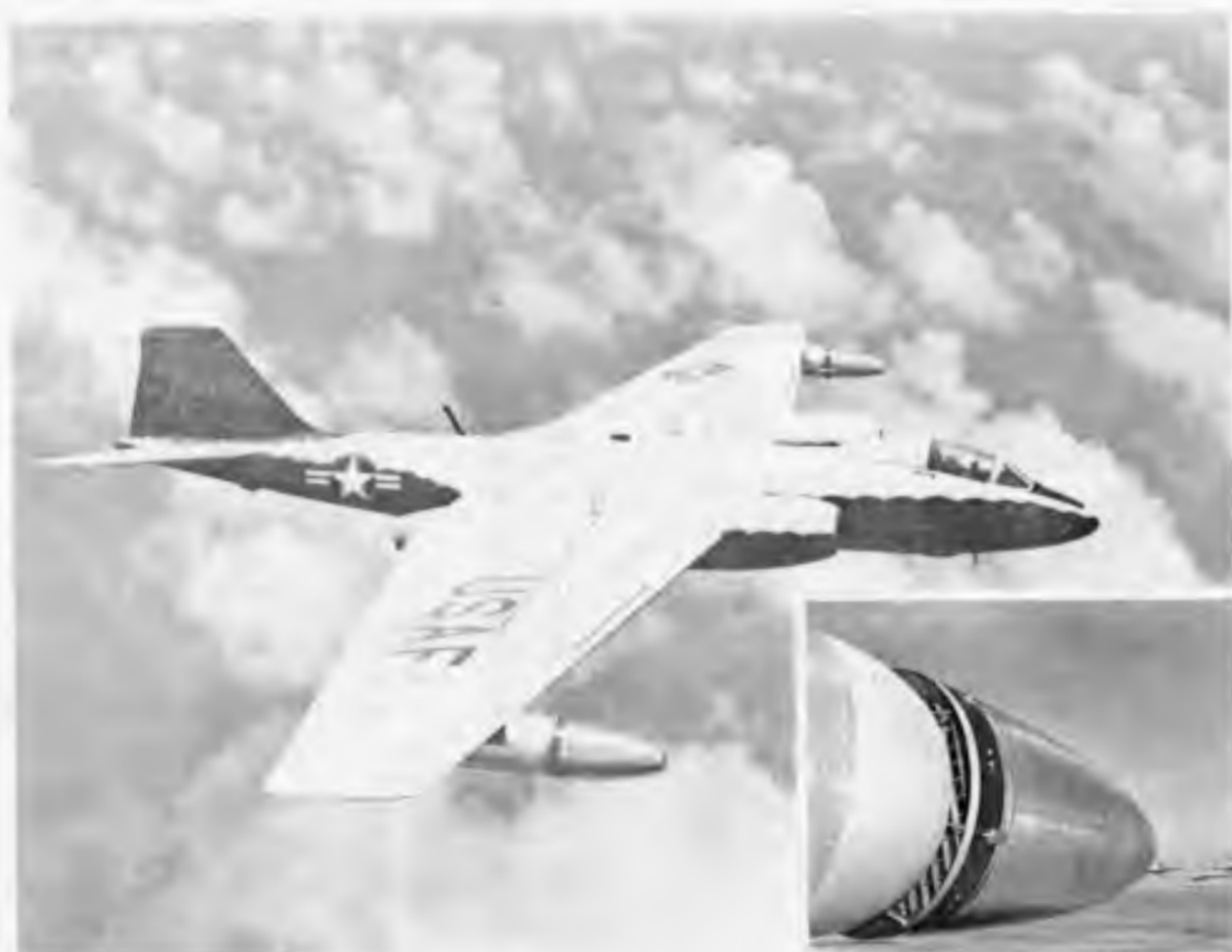
Figure 28. B-57D sampler, HARDTACK; close-up view of collection filter unit inset.
