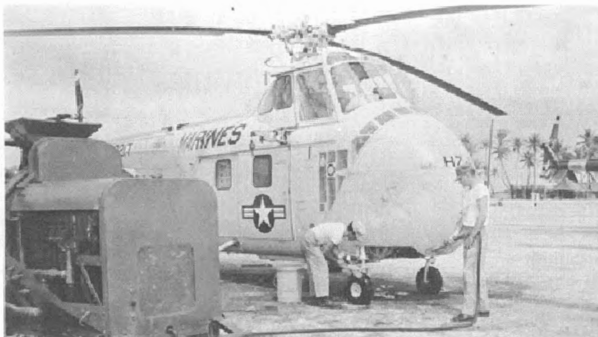
Figure 29. Scrubbing helicopter to remove contamination, REDWING.
