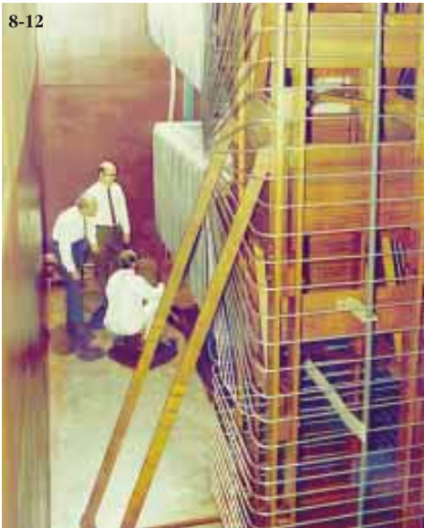
Construction of BLACKJACK radiation test simulator.
