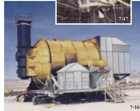
DoD satellite test chamber (HURON KING). INSET: Satellite suspended inside test chamber.
