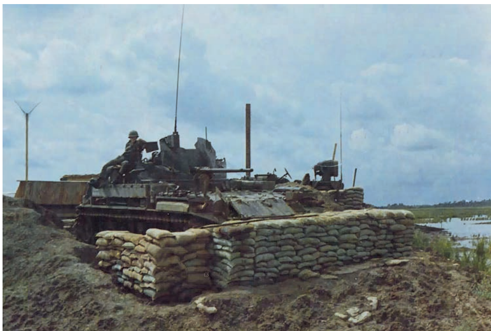
An M42 40-mm. self-propelled antiaircraft gun, or "Duster," provides perimeter defense.
