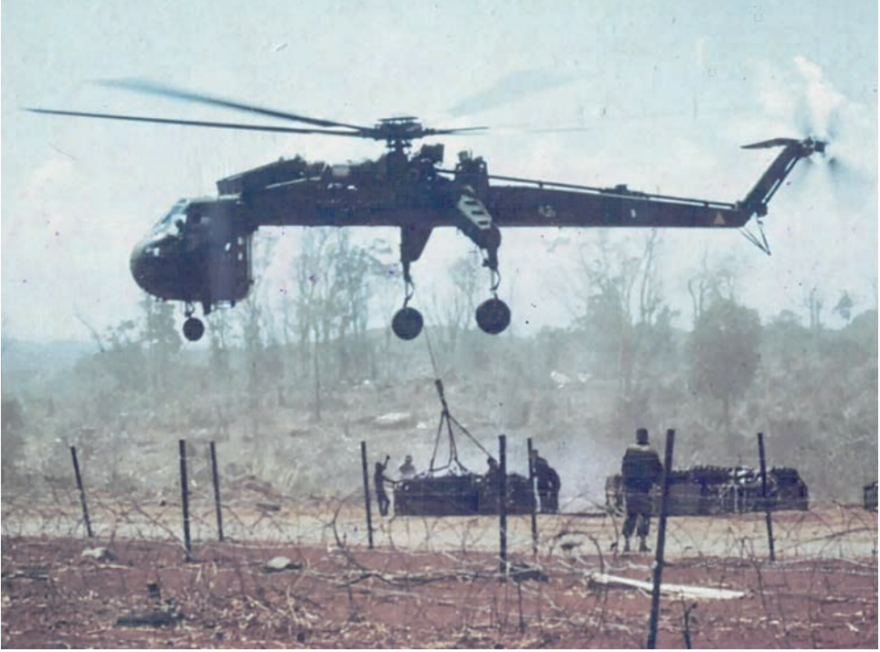
A CH-54 Tarhe, or Flying Crane, picks up a sling load.
