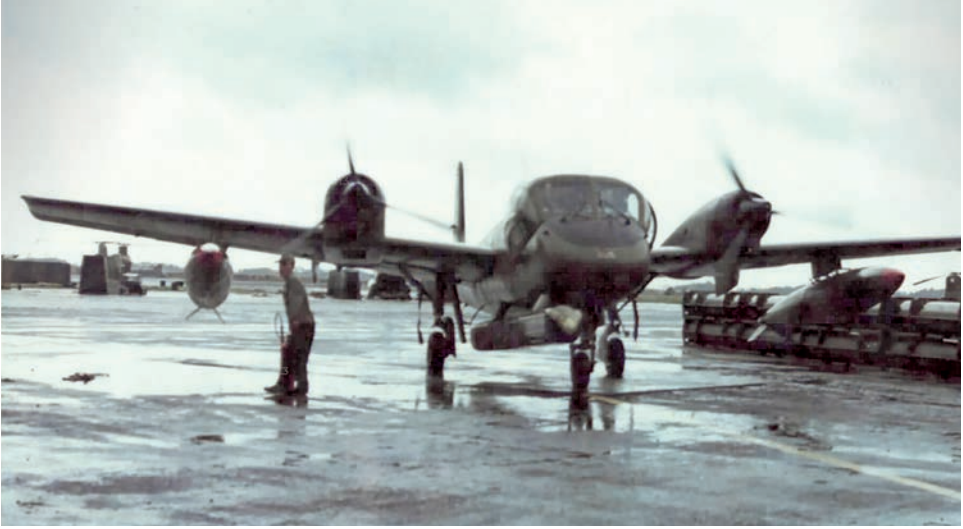
An OV-1B Mohawk surveillance aircraft equipped with a side-looking airborne radar pod
