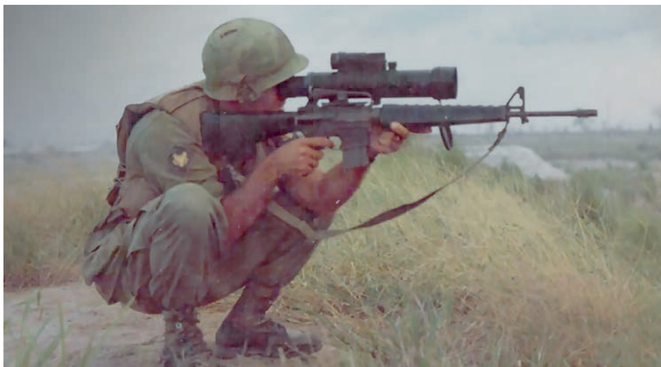
A soldier looks through an AN/PVS-2 Starlight scope mounted on top of an M16 rifle.
