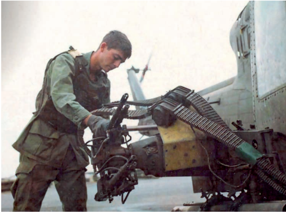
A crewman from the 4th Platoon, 120th Aviation Company, checks the twin side-mounted M60 machine guns on his Huey gunship at Tan Son Nhut.
