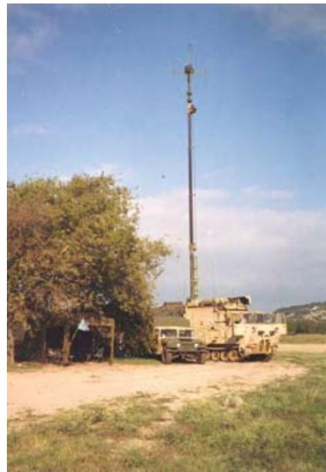
*AN/TSQ-138 Trailblazer, a Mobile, Ground-based Electronic Warfare Signals Intelligence Intercept System. As a tactical direction-finding and intercept system to provide support to the tactical commander, it performs many of the former functions of the Apache Scouts.*
