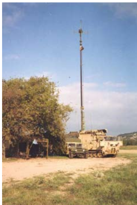
AN/TSQ-138 Trailblazer, a Mobile, Ground-based Electronic Warfare Signals Intelligence Intercept System. As a tactical direction-finding and intercept system to provide support to the tactical commander, it performs many of the former functions of the Apache Scouts.
