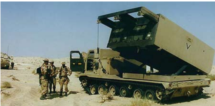
Multiple Launch Rocket System (MLRS) Deployed during DESERT STORM, 1990–1991. The NCOs of today are responsible for the greatly intensified lethality of artillery on the battlefield, which is now able to blanket a square kilometer in less than a minute.
