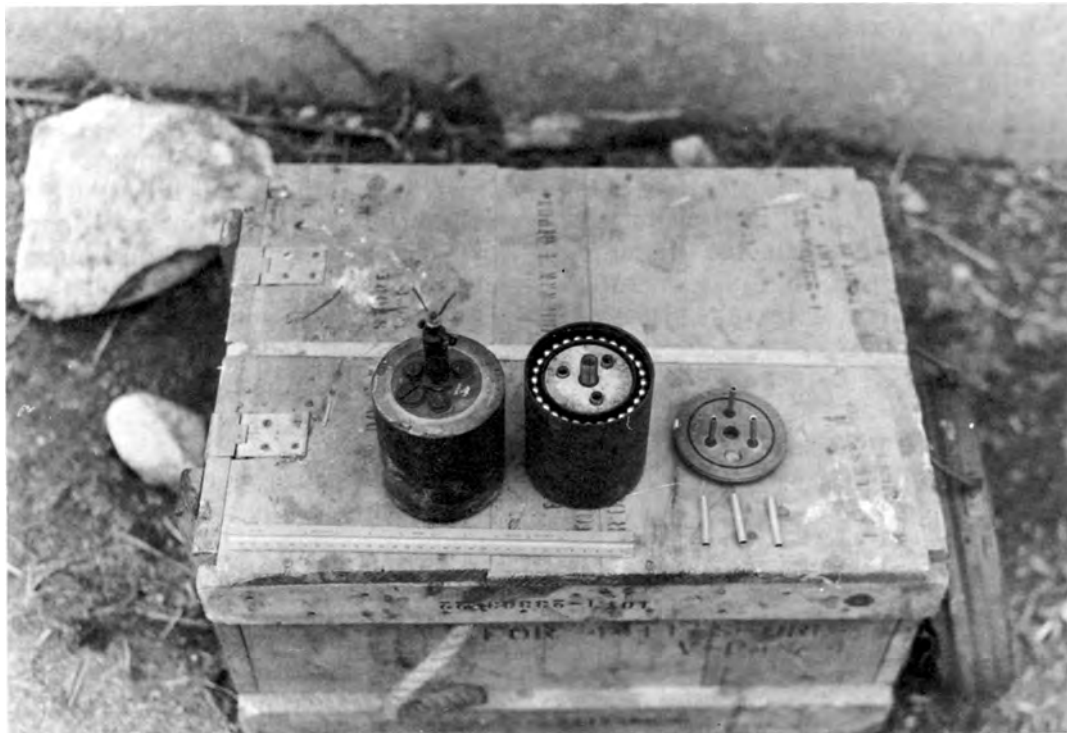
GERMAN S-MINE. The activated canister burst from the earth and fired over 300 steel pellets in all directions.
