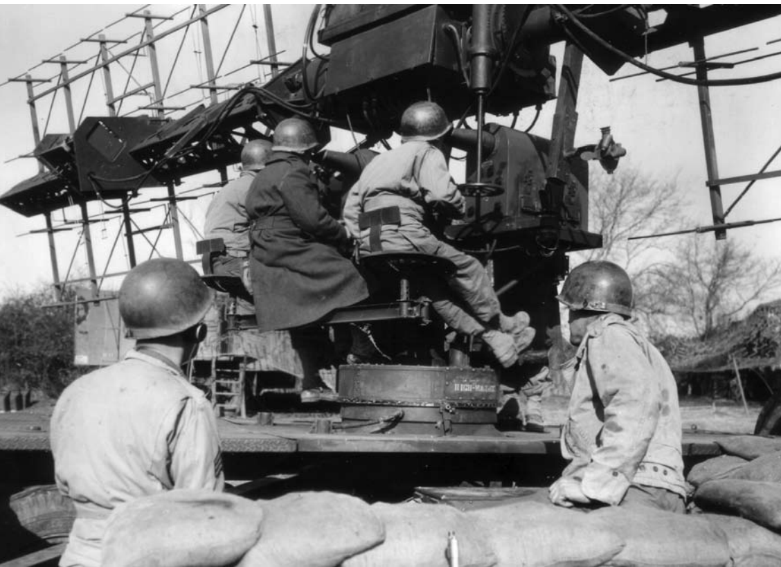
Soldiers of the 68th Coast Artillery man an SCR-268 radar set at the Anzio beachhead in Italy in February 1944. The ability to deploy mobile radar sets with troops in the field helped defeat enemy airpower during World War II. ( National Archives )
