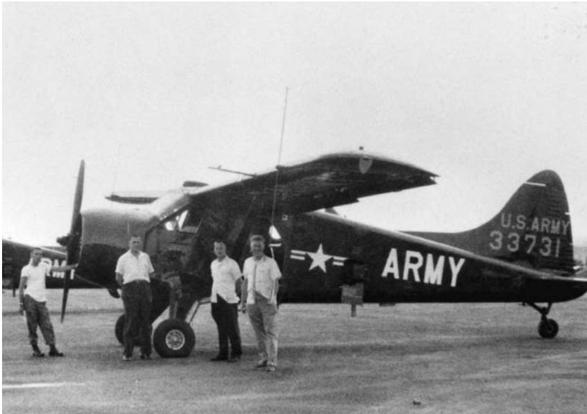
At a Saigon airfield Herbert S. Hovey Jr. ( second from left ) and other engineers stand in front of a U-6 equipped with the first operational radio direction-finding set. The vertical dipole antenna is visible on the near wing. ( Harold Jaffe / U.S. Army Intelligence and Security Command )
