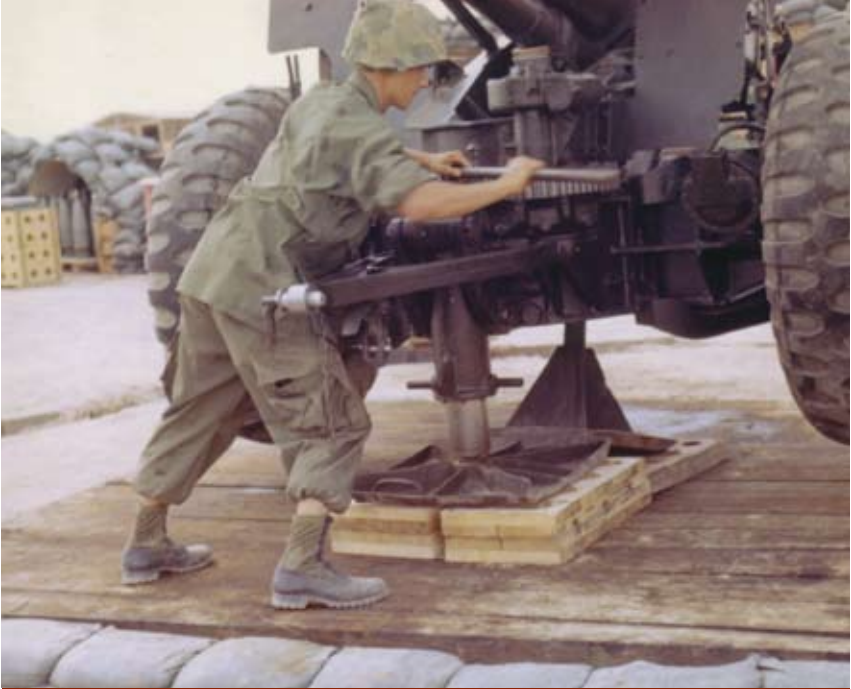
An artilleryman raises the firing jack ( front ) to lower the gun onto the speed jack ( rear ). The latter device was simple, and artillery batteries fabricated them in Vietnam as the concept spread throughout the war zone. ( National Archives )
