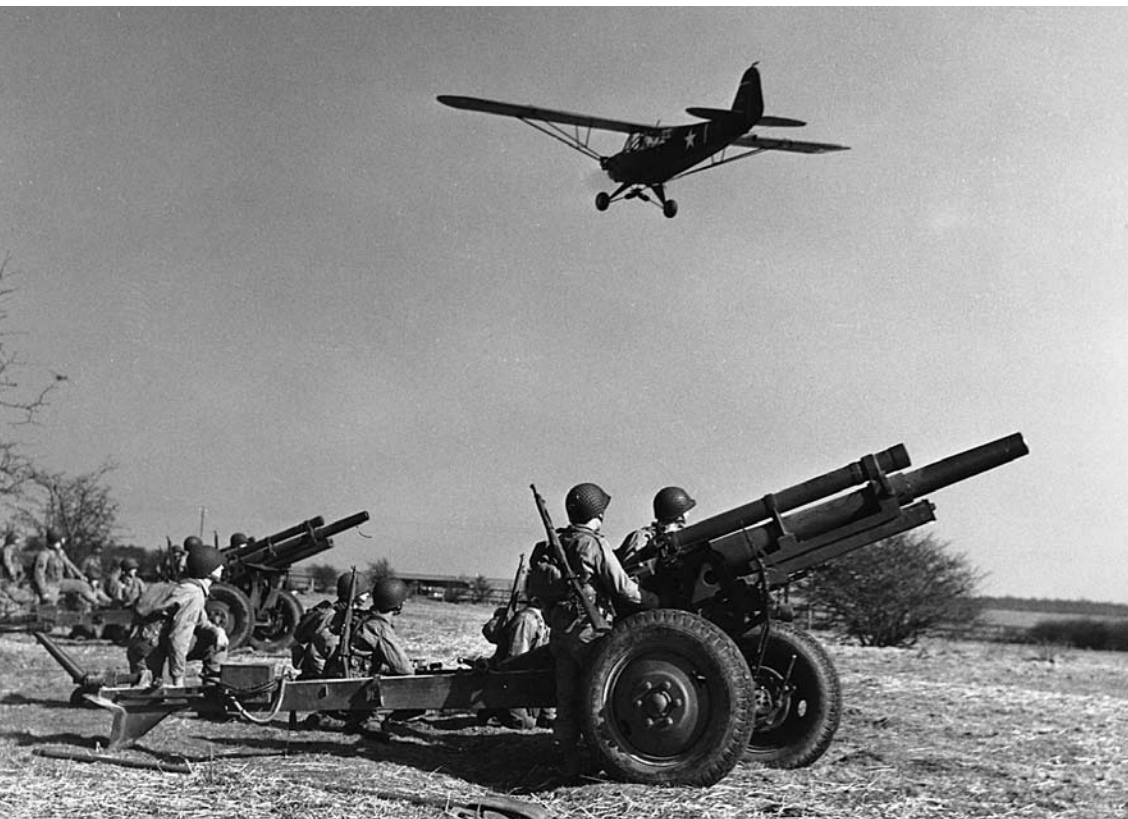
An L-4 of the 29th Infantry Division flies over a battery of M2 105-mm. howitzers in England in March 1943. The integration of light aircraft into artillery units increased the effectiveness of indirect fire. ( National Archives )
