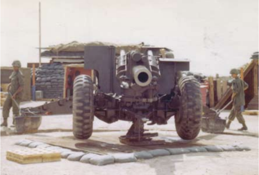
Two soldiers easily maneuver their six-ton howitzer into firing position. The speed jack saved precious seconds in providing fire support to troops in contact. ( National Archives )
