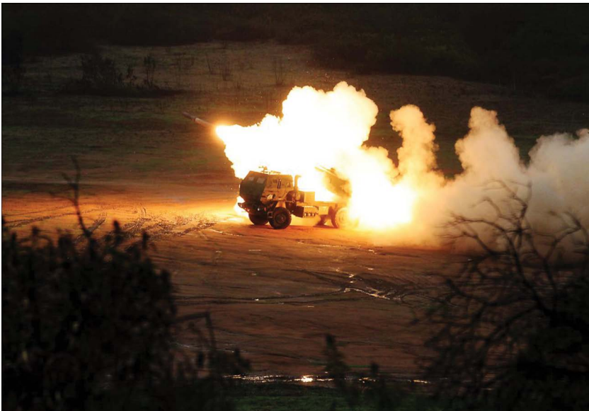
Figure 7.5. M142 High-Mobility Artillery Rocket System (HIMARS). Department of Defense photo by Lance Cpl. Joseph Scanlan.
