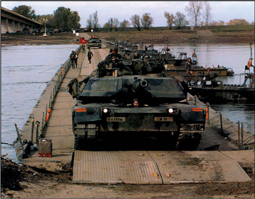
Figure 10.5. Tanks cross a river on a float bridge during brigade training exercises. Courtesy of US Army.
