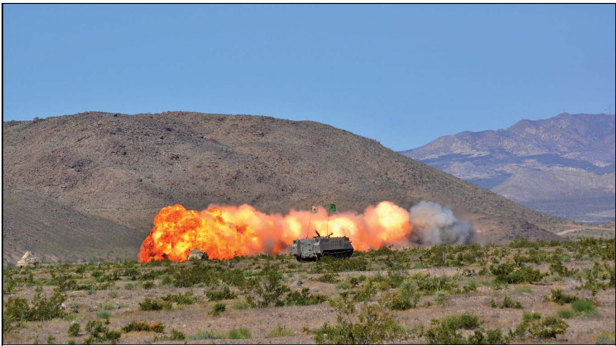
Figure 12.2. Engineers from the 10th Engineer Battalion detonate a mine clearing line charge to allow 3rd Battalion, 69th Armor Regiment to breach an obstacle during a 13 April 2017 live-fire exercise at the National Training Center, Fort Irwin, California. US Army photo by Maj. Randy Ready.
