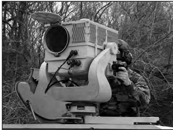
Figure 99. Close-up view of the LRAS3, which greatly increased the scout's ability to see the battlefield.
