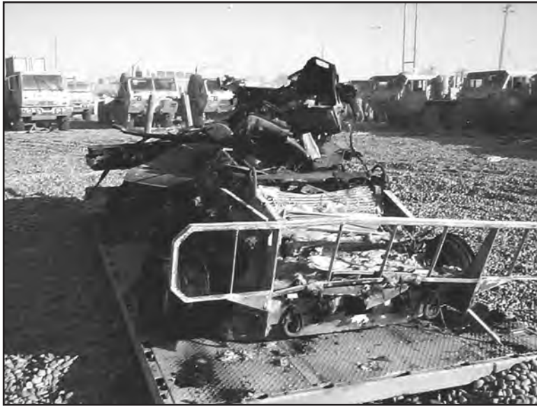
Figure 125. Remains of a HMMWV after an IED attack.
