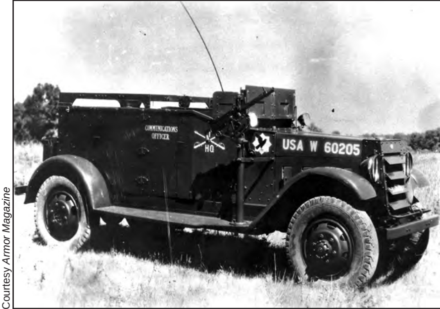
Figure 5. M1 Scout Car, distinguishable from armored cars by its open top and limited armor protection.
