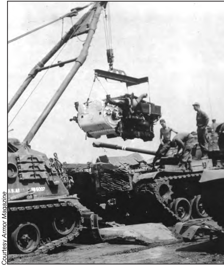
Figure 65. Replacing the M48's engine in the field.
