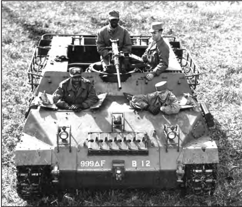
Figure 41. The M39 Armored Personnel Carrier, initially developed at the close of World War II and based on the chassis of the M-18 Gun Motor Carriage.
