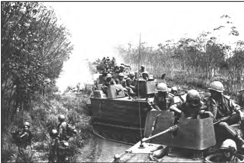
Figure 61. Modified through the addition of machineguns and the installation of gun shields, the M113 became transformed into the Armored Cavalry Assault Vehicle (ACAV).
