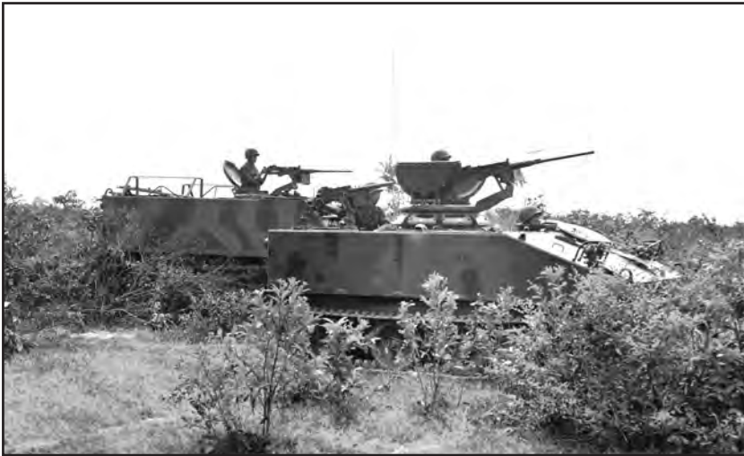
Figure 57. The M114 Armored Command and Reconnaissance Vehicle (foreground) fielded with great promise as a replacement to the venerable jeep.
