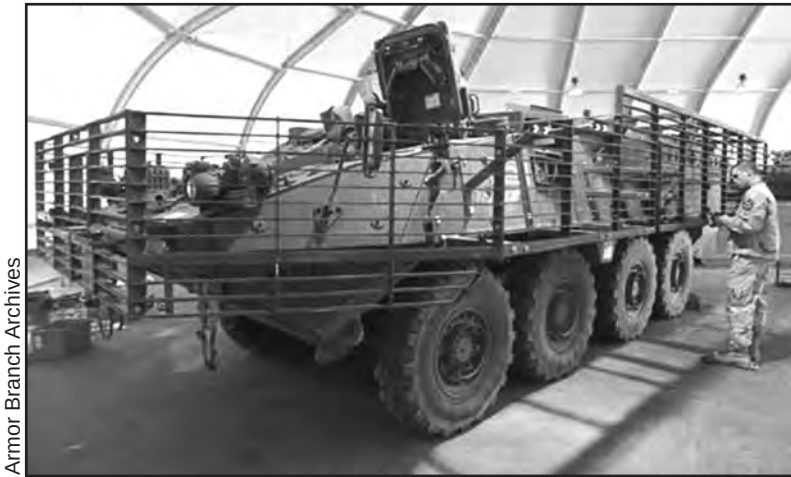
Figure 131. Stryker with slat armor installed to provide improved protection against RPGs.
