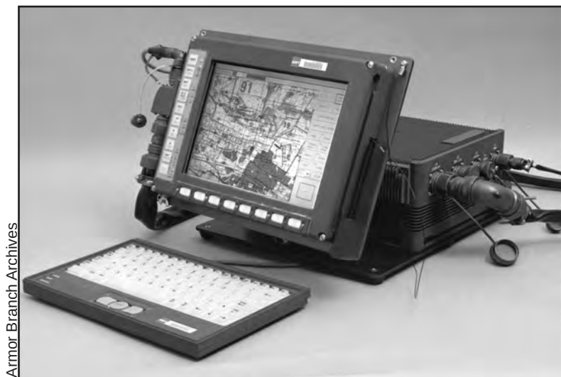
Figure 105. The basic components of the FBCB2.
