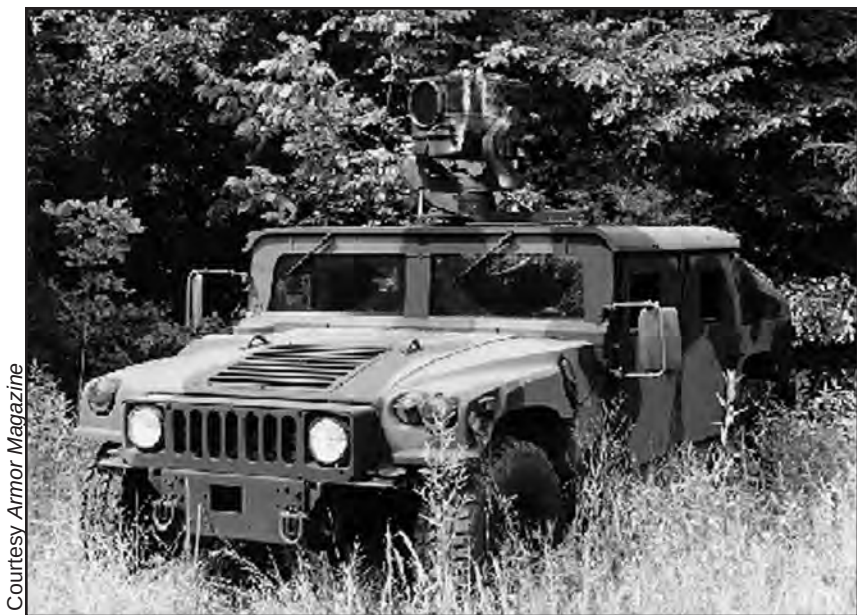
Figure 103. The LRAS3-equipped HMMWV was intended for fielding in the new brigade reconnaissance troop.
