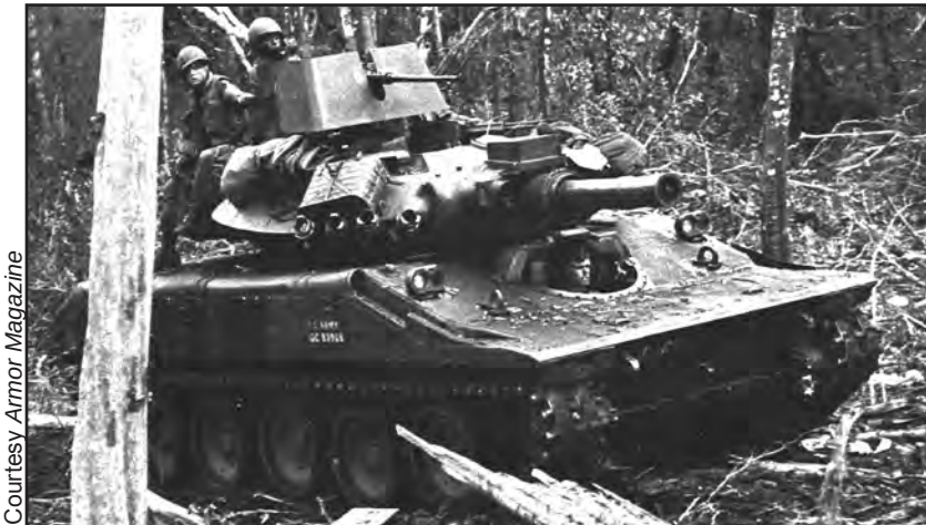
Figure 74. Sheridan with added protection for the tank commander against small arms fire and snipers.
