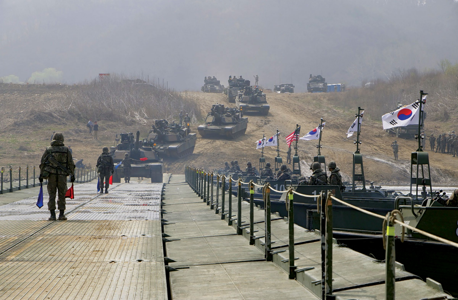
Soldiers drive 68-ton M1A2 Abrams main battle tanks and 27-ton M2A3 Bradley infantry fighting vehicles across a floating bridge over the Imjin River 8 April 2016 near Seoul, South Korea. The Imjin River is the seventh-largest river in Korea and flows from North Korea into South Korea across the Demilitarized Zone. Soldiers from the 2nd Battalion, 8th Cavalry Regiment, 1st Armored Brigade Combat Team, 1st Cavalry Division, crossed the bridge assembled by the Republic of Korea Army 6th Engineer Brigade as part of a four-day, combined arms river crossing exercise. (Photo by Sgt. Christopher Dennis, U.S. Army)
