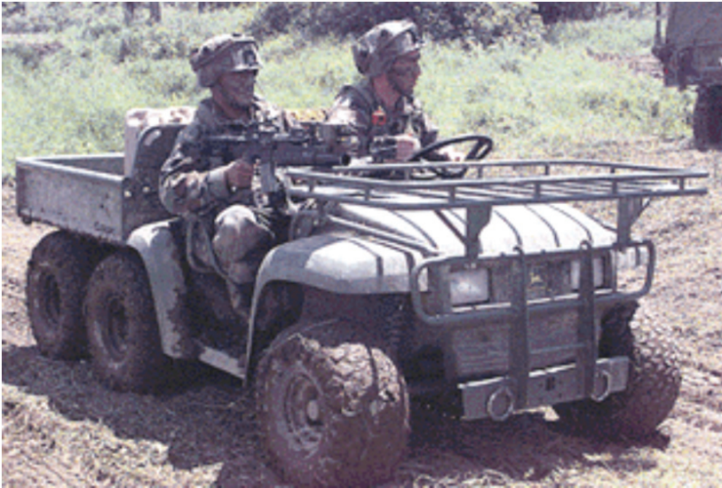
Figure 12. The Military Gator. This is a two-seat, six-wheel squad vehicle that can carry up to a 550-kg load and runs on JP8 fuel.
