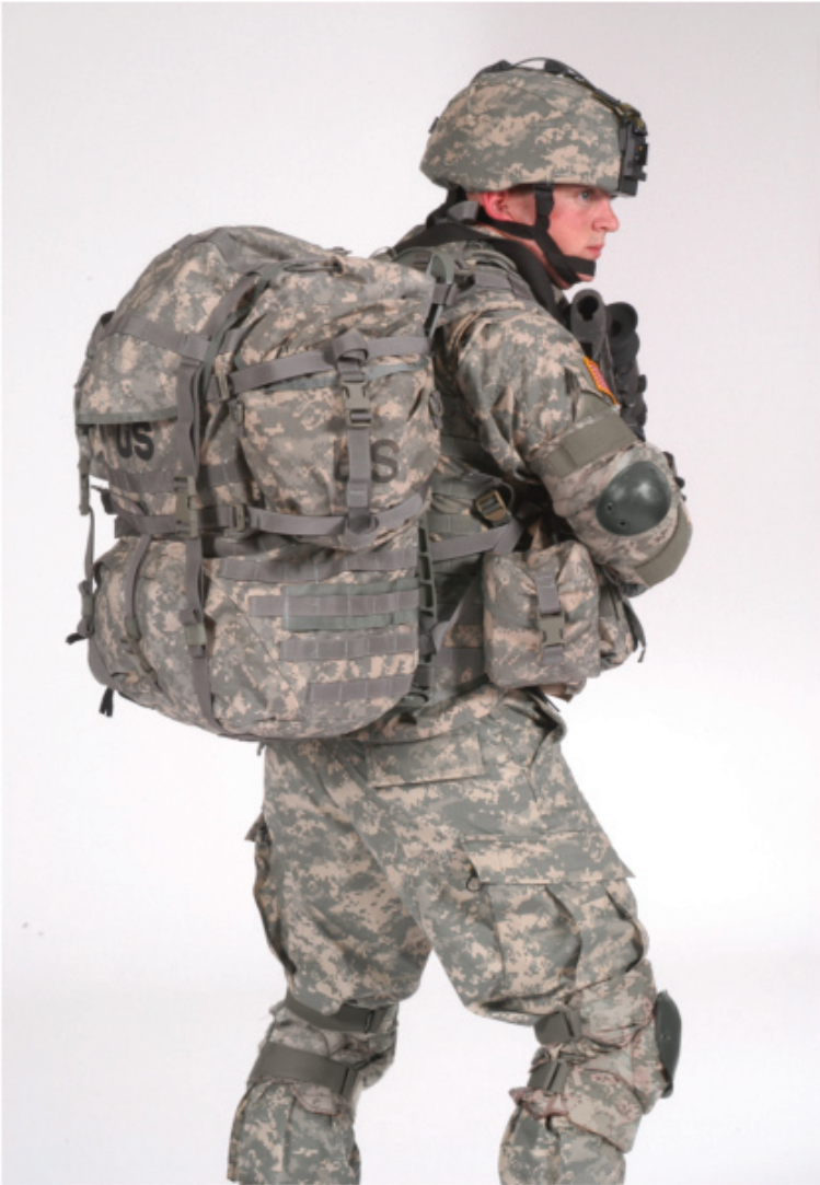
Figure 8. Soldier wearing the Modular Lightweight Load-Carrying Equipment (MOLLE) pack. The MOLLE pack is an entire modular system that includes a main pack with an external frame, butt pack, and load-bearing vest. A patrol pack can be detached and used separately. The vest has removable pockets to accommodate different objects. Padded shoulder straps, waist belt, and strap adjustments allow for better load distribution, and the soldier can shift the load to different anatomical locations.
