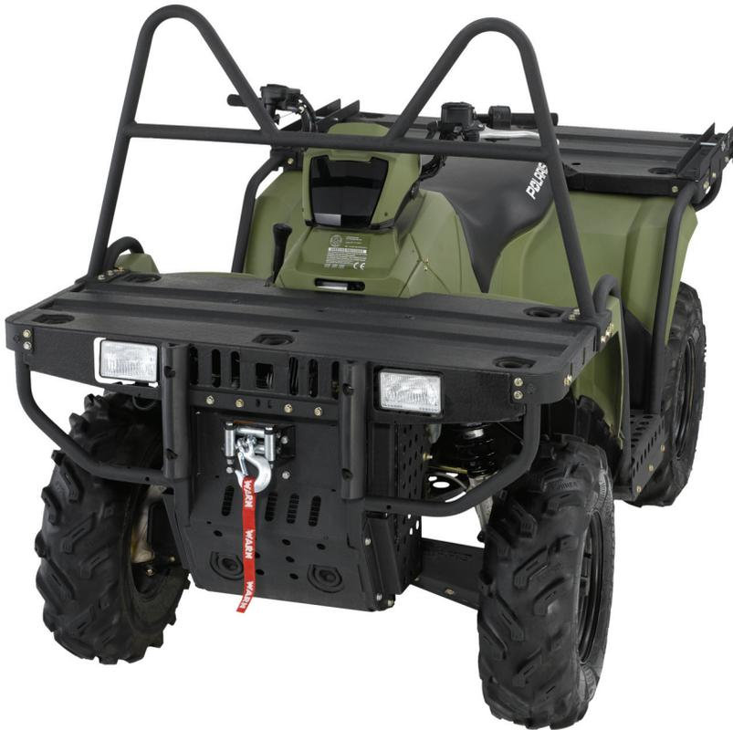
**Figure 14.** Polaris Sportsman military vehicle. It is a four-wheel, all-terrain vehicle that can carry one person and a load up to 204 kg.
