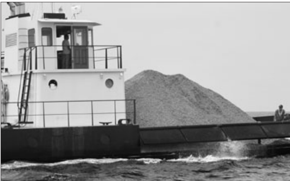
Ground-up shells being deposited in the Delaware Bay in 2005 to promote oyster habitat and help restore the native oyster population
