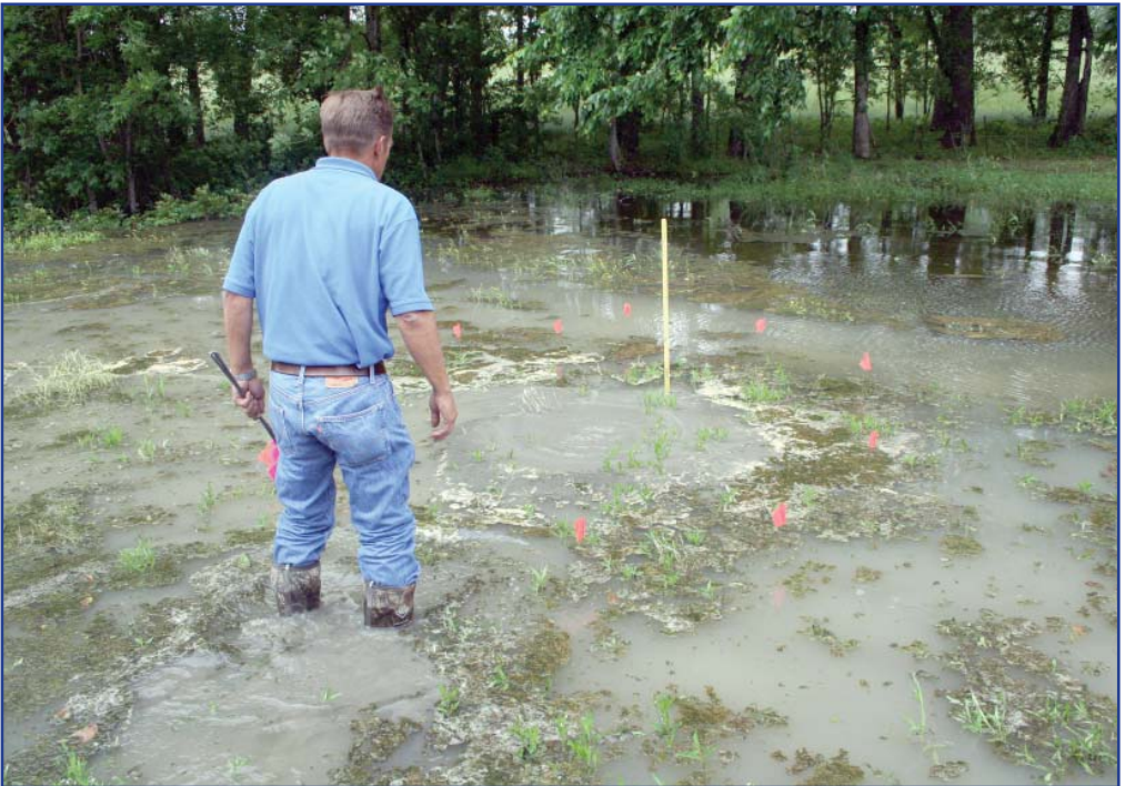
Robert Thompson intently watches the development of a sand boil.
