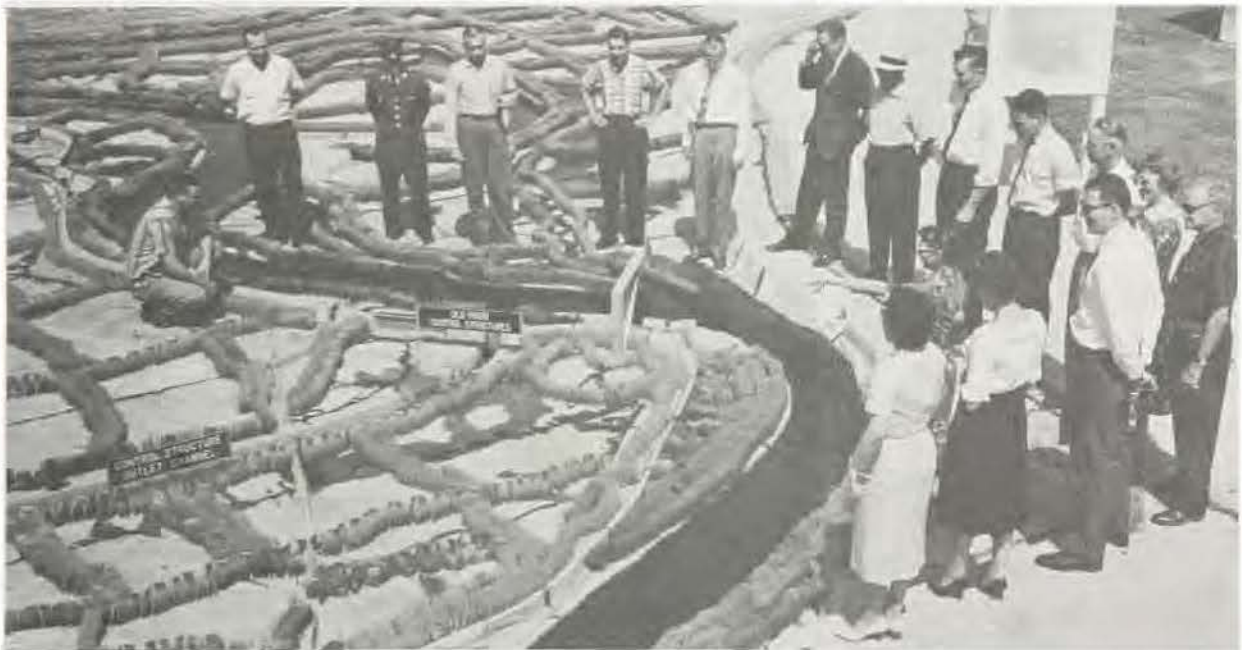
"Old 94"; guide is pointing out the portion of the model used in tests to prevent capture of the Mississippi River by the Atchafalaya River
