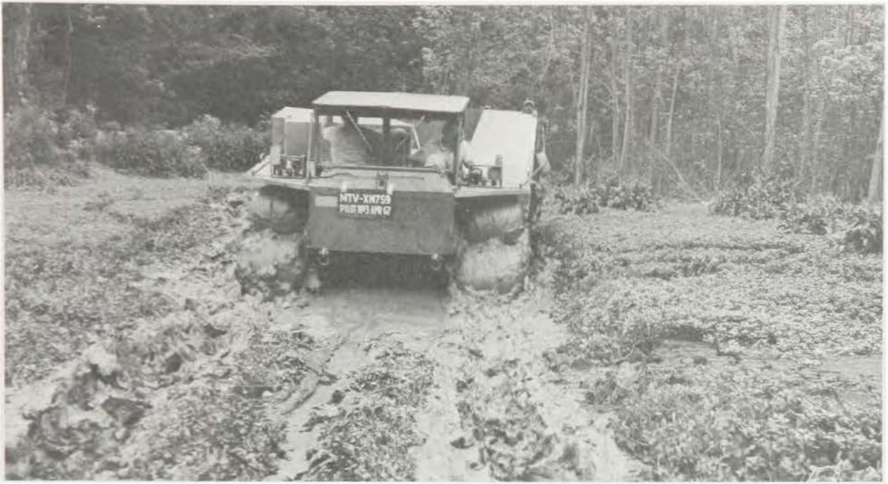
XM759 vehicle operating in extremely soft soil
