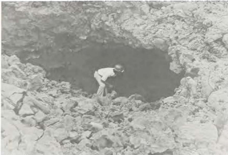
This opening was blasted into a lava tube on the flank of Mauna Loa Volcano. The analysis of tests such as these will help scientists to evaluate potential use of explosive charges to hinder or stop volcanic flows in the event of an eruption on the giant mountain
