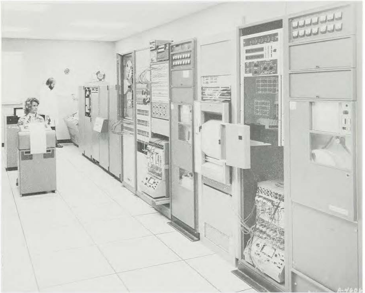
Data reduction equipment which is used for converting analog data so that it may be analyzed for use in the ADP Center and processed for reports, etc.
