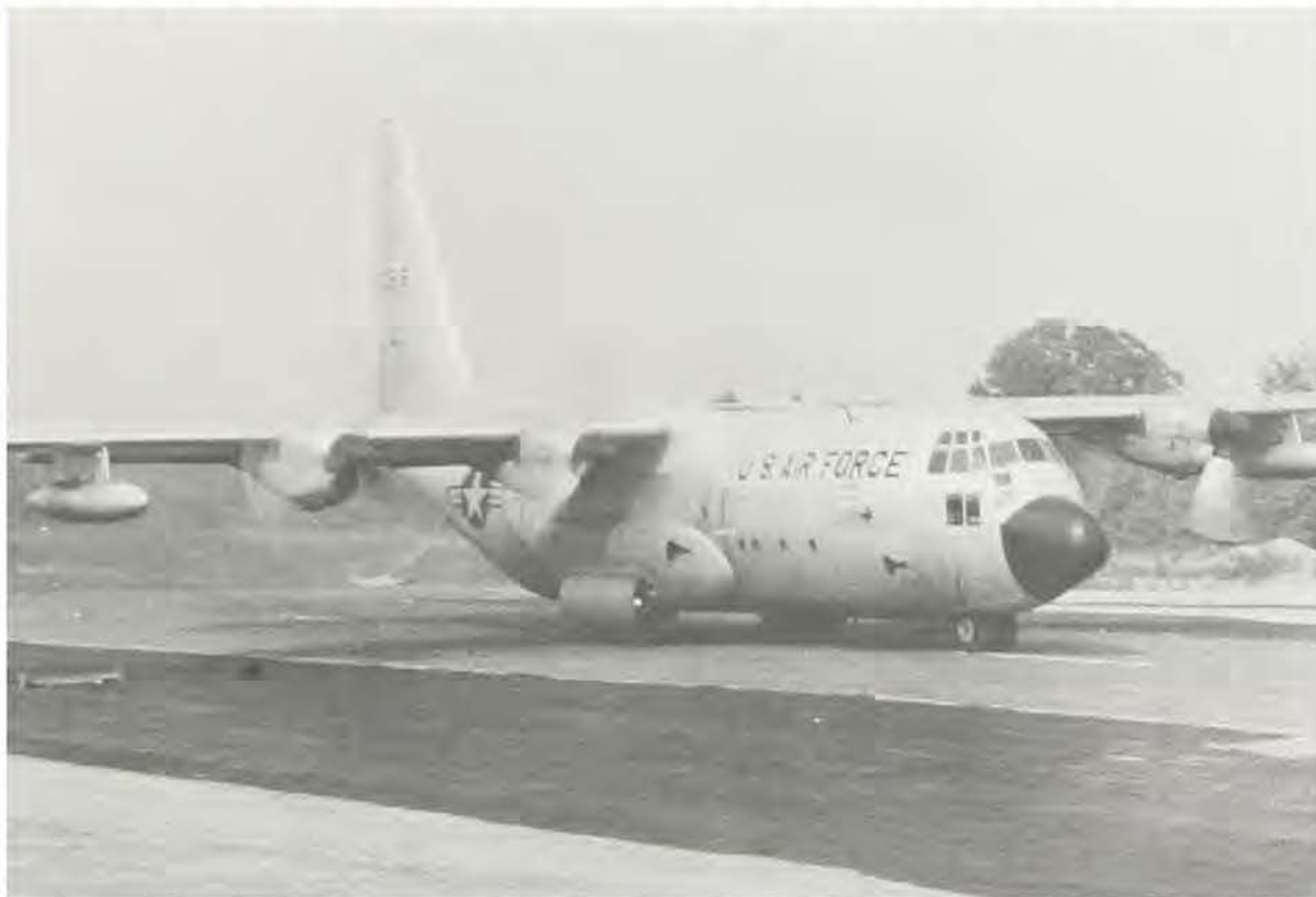
C-130 aircraft operating on membrane-surfaced runway
