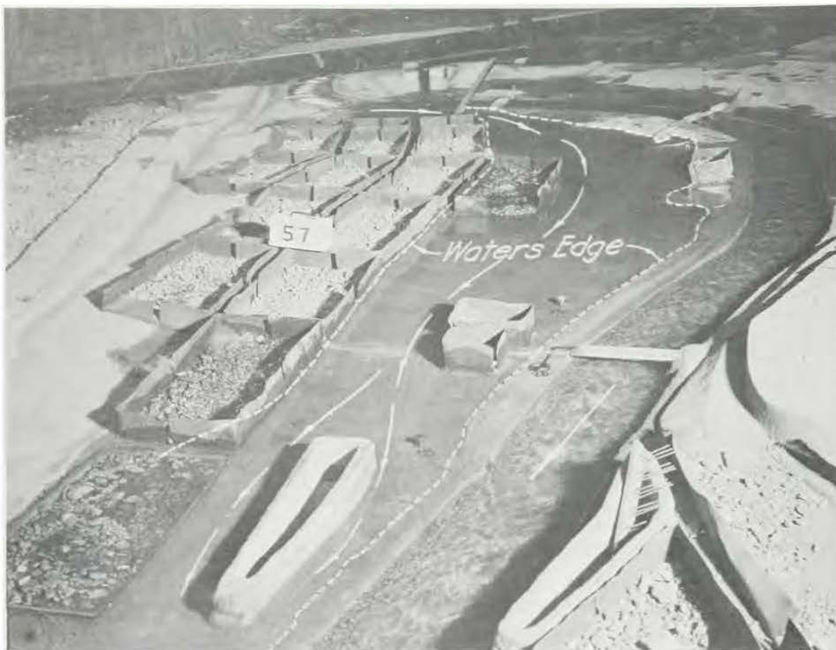
Model used in studies of Johnstown flood control project
