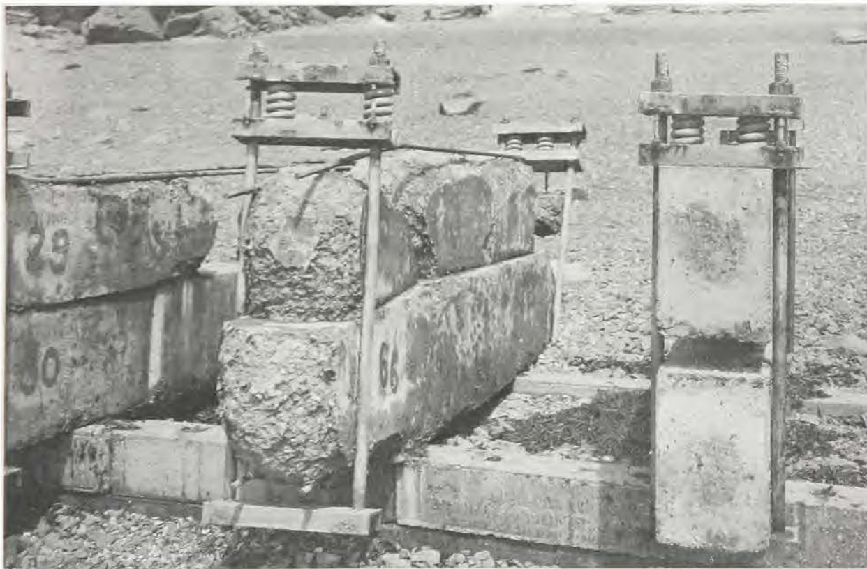
Condition of concrete beams after 1-1/2 years of freezing and thawing cycles and tidal inundation at Treat Island, Maine, weathering station
