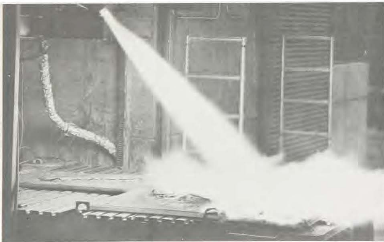
Rocket engine blast test with rocket motor firing on landing mat
