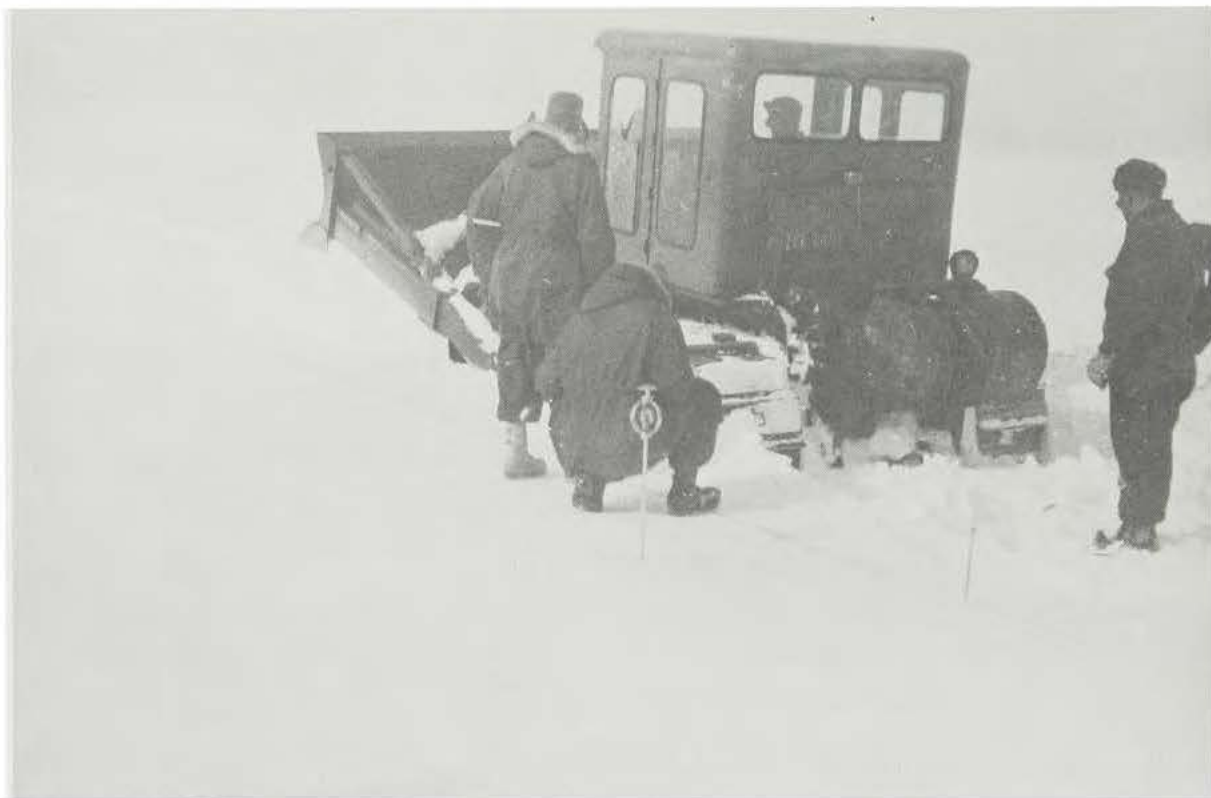
Trafficability testing of standard D-7 Caterpillar tractor on polar ice cap
