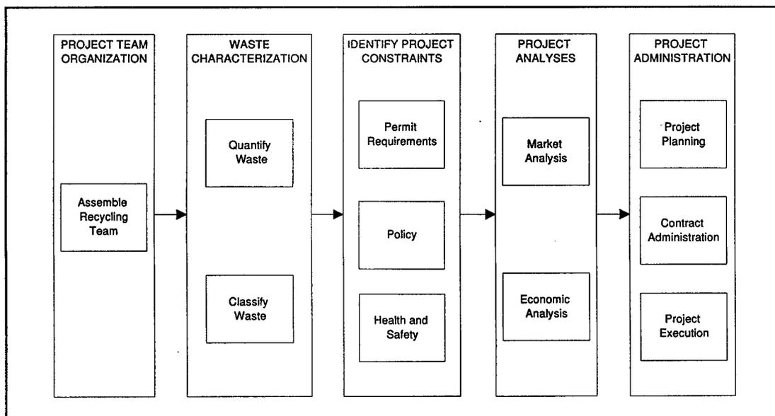
Figure 2. Development of a recycling plan.
