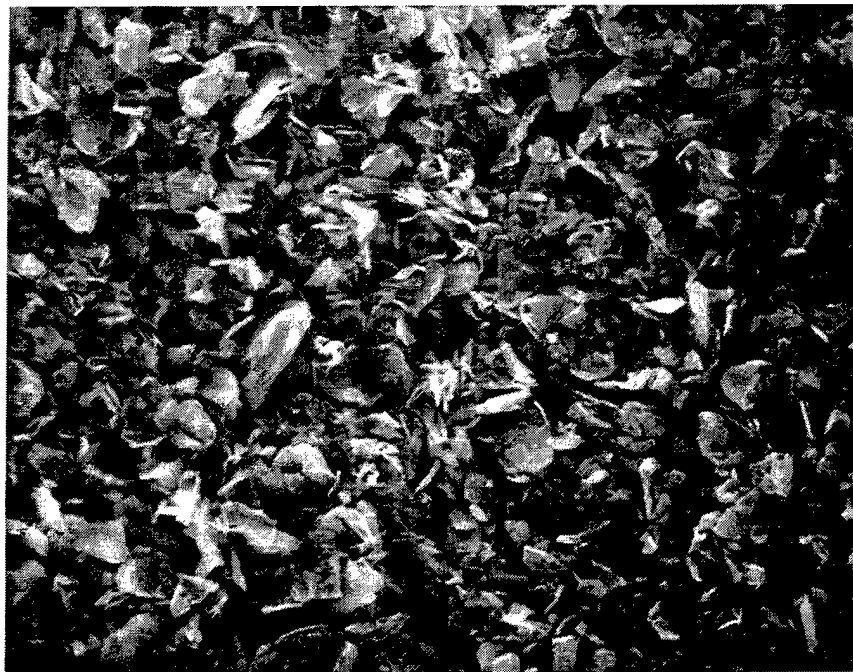
Figure 5. SEM of Natural Graphite Powder.
