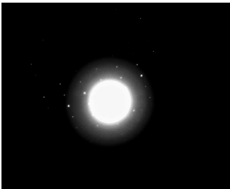
Figure 4. Selected area electron diffraction pattern of the \text{Co}_{0.95}\text{Pd}_{0.05}\text{Te}_{0.05}\text{Sb}_{2.95} alloy after the end of the first discharge/charge cycle.
