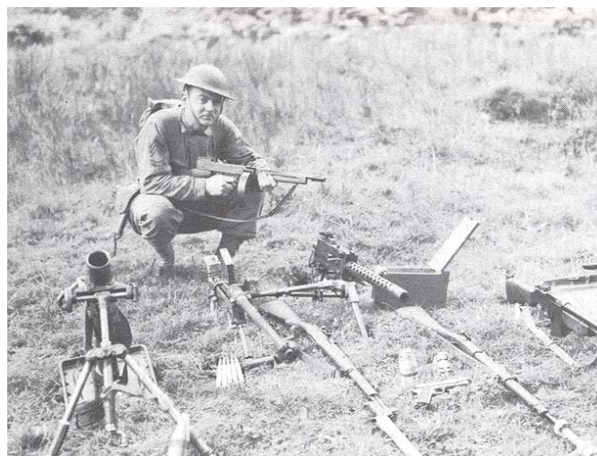
Weapons, left to right: Soldier is holding a .45-cal. Thompson submachine gun M1928A1. 60mm Mortar M2; British Anti-Tank Gun; .30-cal. U.S. Rifle M1 with Bayonet M1; .30-cal. Browning light Machine Gun M1919A4; hand grenades; .45-cal. M1911A1 pistol; .30-cal. U.S. Rifle M1903 with grenade launcher M1; .30-cal. Browning Automatic Rifle M1913A2.
