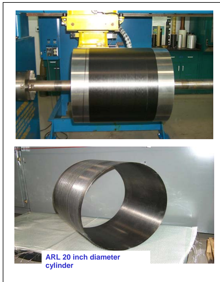
Figure 7. Twenty-inch diameter composite cylinders fabricated at ARL facilities.
