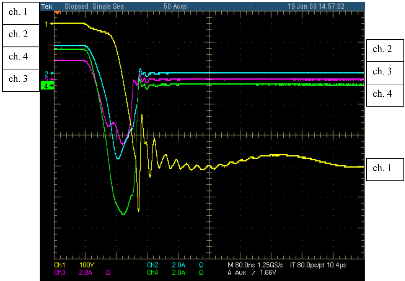
Figure 7. Continuous operation of Cotronics-coated module4 p-i-n in DC-to-DC buck converter.
