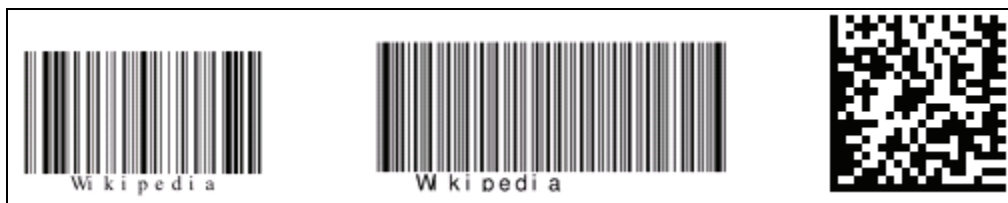
Figure 2.1. Bar code representations of “Wikipedia,” the internet encyclopedia, using a both 1D and 2D (right) configurations
