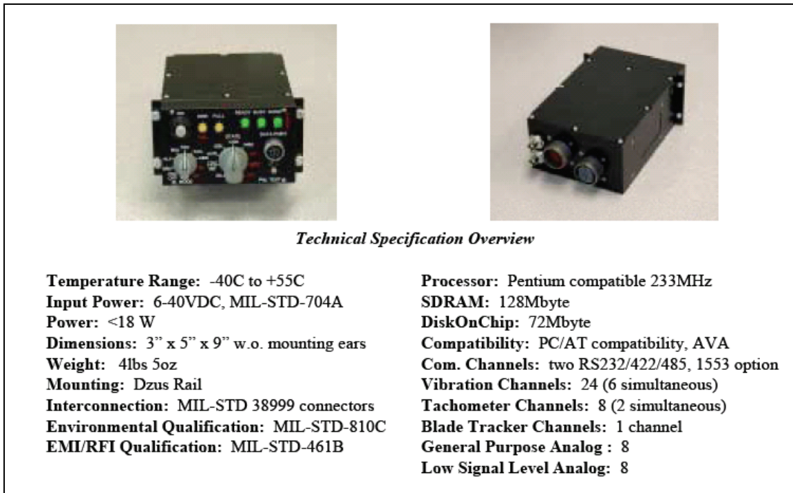
Figure 2.21. Technical specification of the HUMS box for the VMEP.
