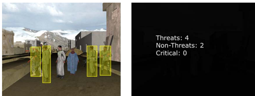
Fig. 13 Robot's report shows its immediate environment is unsafe; (left) in image report 4 threats are bounded in yellow boxes while (right) text report counts the total number of threats
