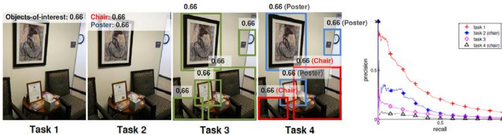
Fig. 30 Task conversion for human perception and precision and recall curve for all 4 tasks. Precision and recall are calculated for Subject 1’s perception ability. For Task 2 and 4, the PR curve for the “chair” category is shown.
