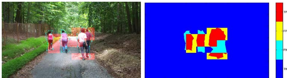
Fig. 45 (left) Classifications (red boxes) overlaid with annotations (cyan lines) and (right) true and FPs and negatives
