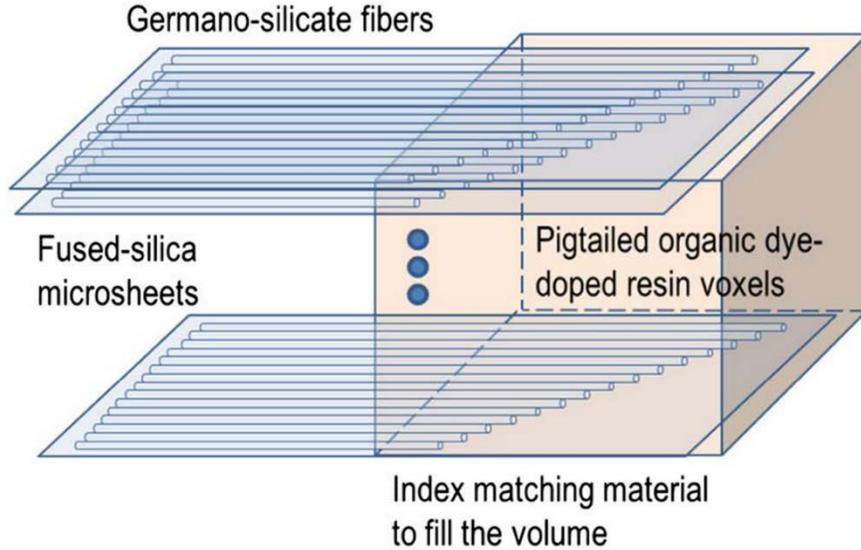
**Fig. 2** Schematic of the optical-fiber-bundle-based static volumetric 3-D display (image reprinted with permission of Geng<sup>4</sup>)
