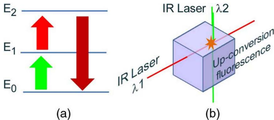
**Fig. 1 Solid-state upconversion: (a) energy-level diagram of an activated ion and (b) 2 intersecting laser beams with different wavelengths are absorbed in ZBLAN (image reprinted with permission of Geng<sup>4</sup>)**
