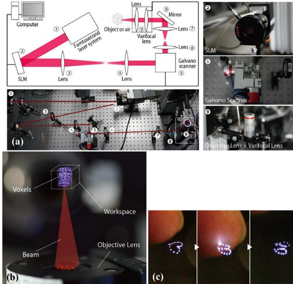
**Fig. 4** (a) Drawing and photograph showing the femtosecond-laser-induced hologram setup where (1) is the femtosecond laser; (2) SLM; (3), (4), (6), and (7) lenses; (5) Galvano scanner, (8) mirror, and (9) the objective and the varifocal lens. (b) Photograph showing the projected voxels with illustrations showing the voxel area and the beam emitting the plasma. (c) Rendered heart that, once touched, splits into 2 ovals. (Images reprinted with permission of Ochiai et al.<sup>19</sup>)
