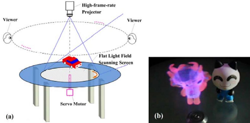
**Fig. 5** (a) Light-field display and (b) resulting holograph of a pink doll next to a real panda figure (images reprinted with permission of Xia et al.<sup>23</sup>)
