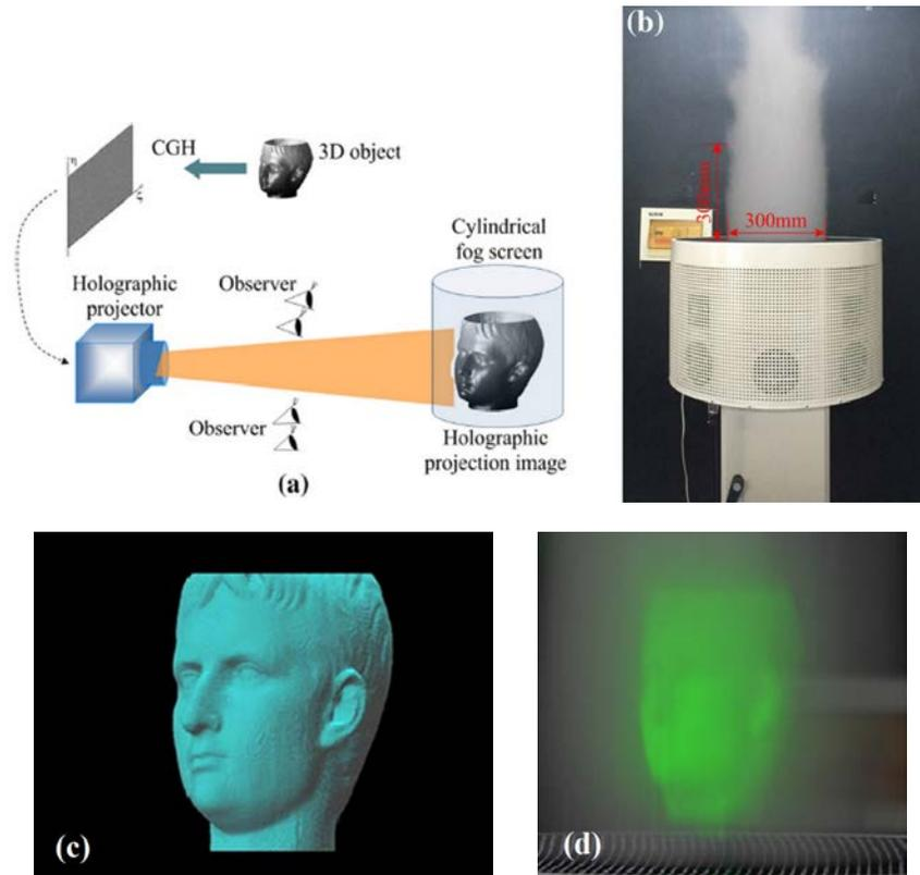
**Fig. 3 Volumetric display: (a) schematic, (b) cylindrical fog-screen apparatus, (c) CGH image, and (d) rendered holographic image (images reprinted with permission of Zeng et al.<sup>17</sup>)**
